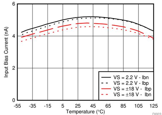
Figure 6-2. Input Bias Current vs Temperature
