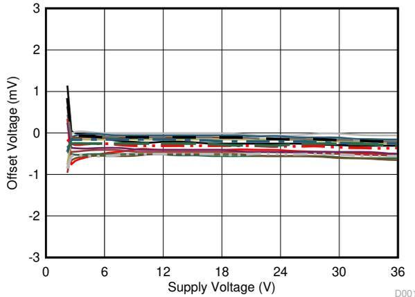
Figure 6-7. Offset Voltage vs Supply Voltage
