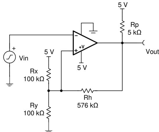
**Figure 8-1. Comparator Schematic With Hysteresis**
