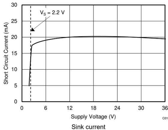
Figure 6-17. Short-Circuit Current vs Supply Voltage
