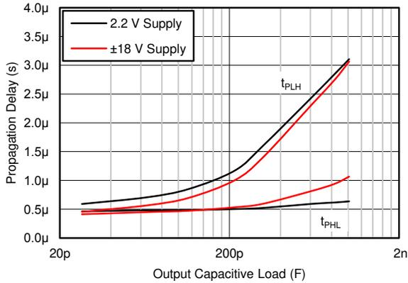
Figure 6-9. Propagation Delay vs Capacitive Load
