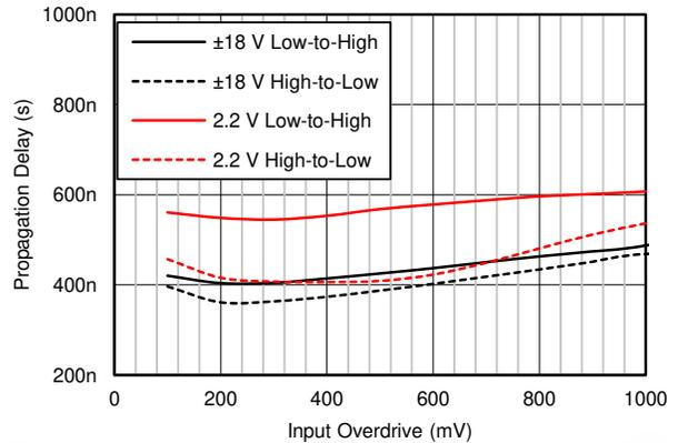
Figure 6-8. Propagation Delay vs Input Overdrive
