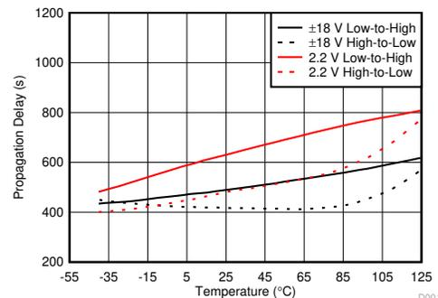
Stable Propagation Delay vs Temperature
