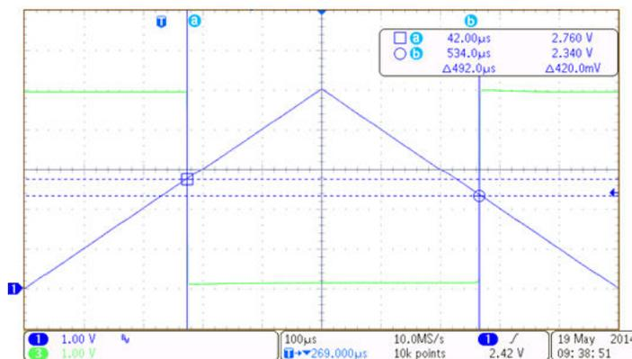
Figure 8-2. TLV1701 Upper and Lower Threshold With Hysteresis
