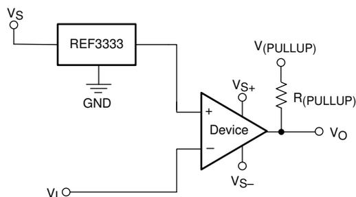
**Figure 7-2. Reference Voltage for the TLV1704-SEP**
