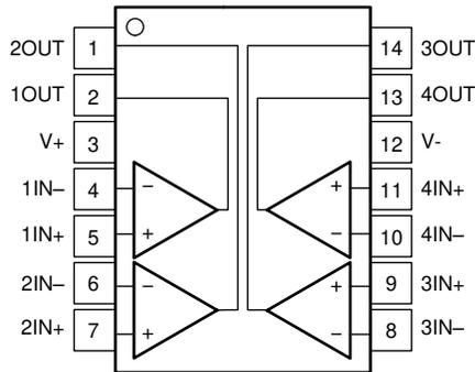
**Figure 5-1. TLV1704-SEP PW Package 14-Pin TSSOP Top View**
