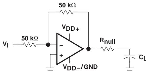
**Figure 60. Series-Resistance Circuit**
