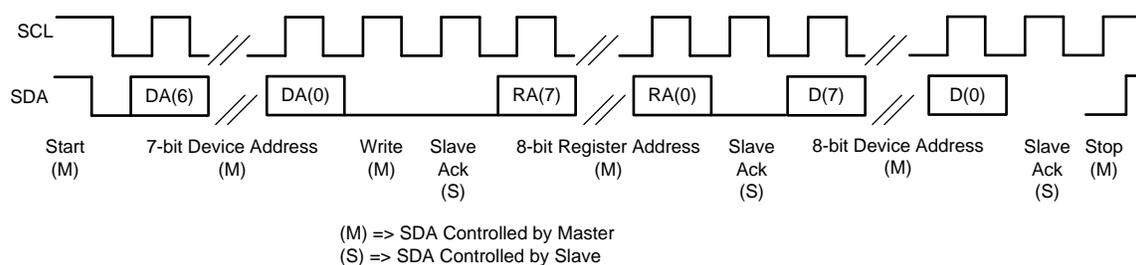
Figure 43. I<sup>2</sup>C Write
