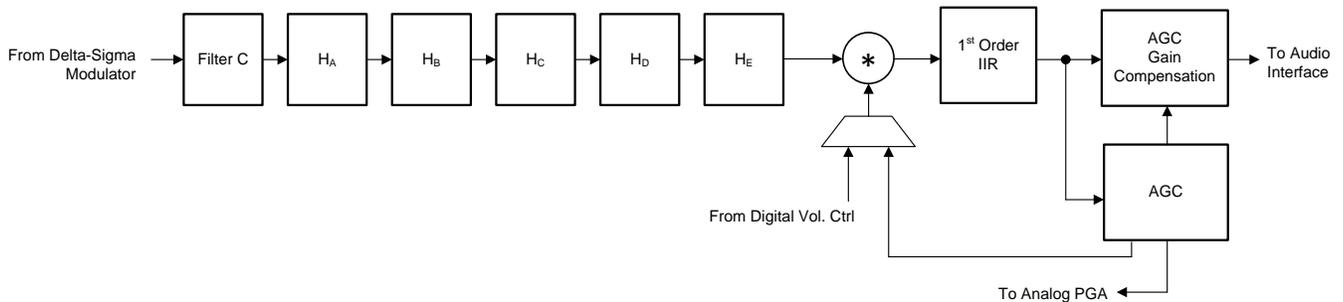
Figure 37. Signal Chain for PRB\_R14 and PRB\_R17
