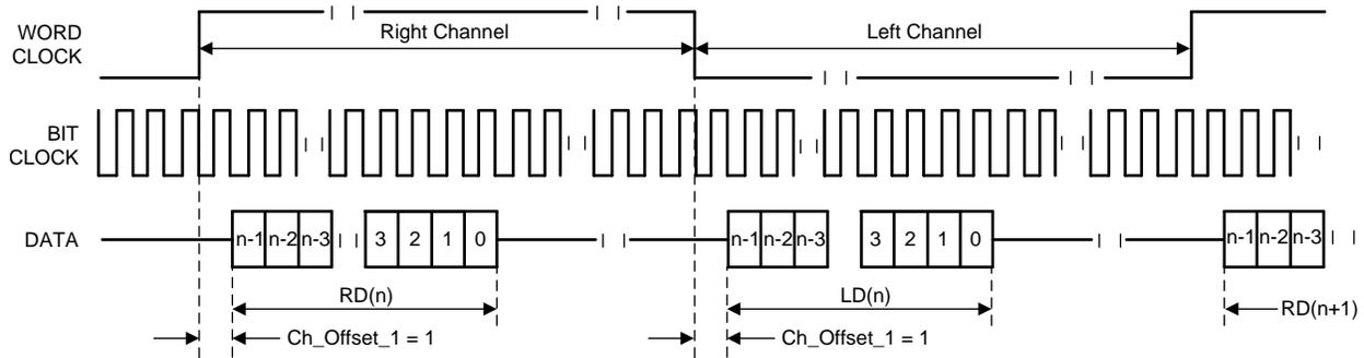
Figure 16. Left-Justified Mode With Ch\_Offset\_1 = 1, Channel Swapping Enabled
