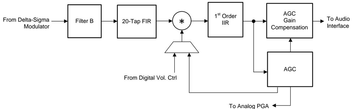
Figure 35. Signal Chain for PRB\_R9 and PRB\_R12
