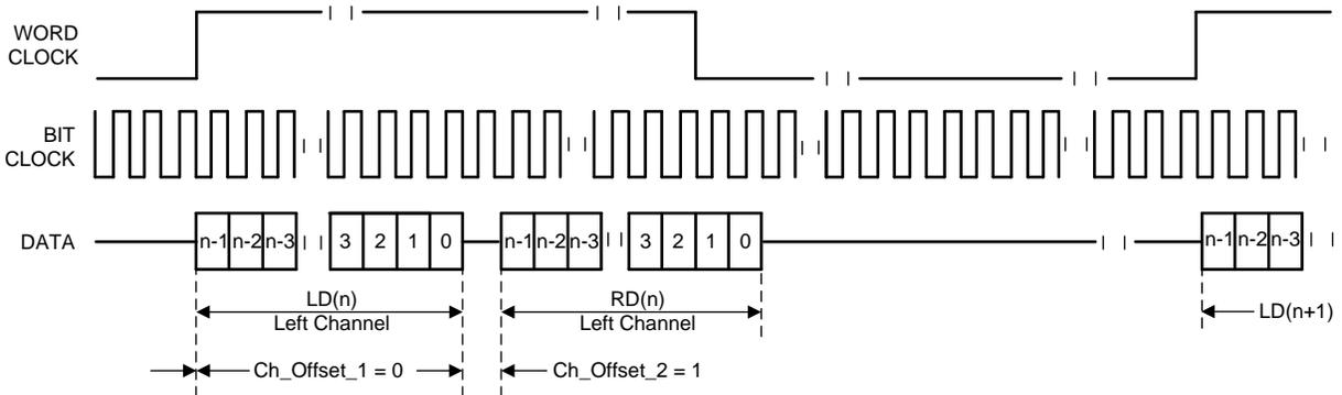
Figure 17. Left-Justified Mode, Time-Based-Slot Mode Enabled, Ch\_Offset\_1 = 0, Ch\_Offset\_2 = 1
