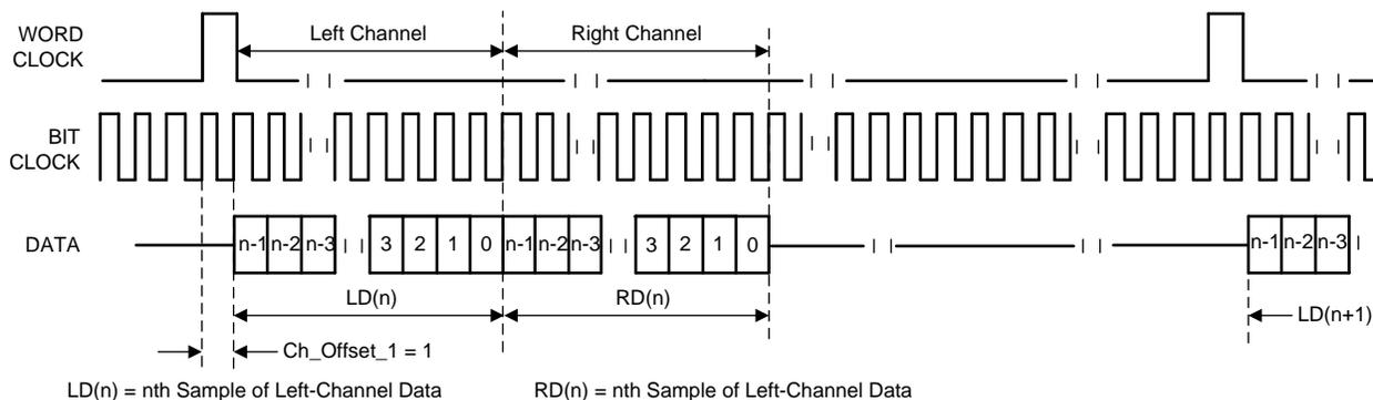
Figure 23. DSP Mode With Ch\_Offset\_1 = 1
