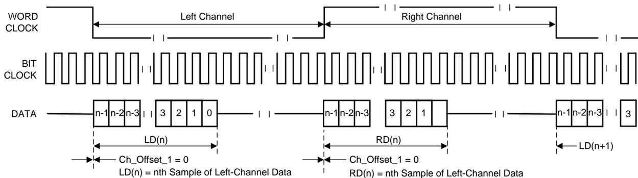
**Figure 19. I<sup>2</sup>S Mode (Standard Timing)**
