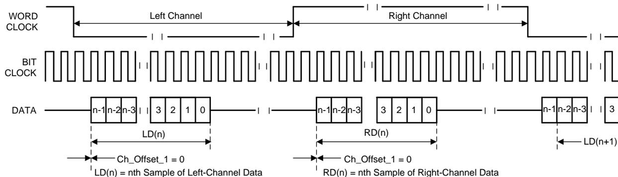
Figure 21. I<sup>2</sup>S Mode With Ch\_Offset\_1 = 0, Bit Clock Inverted
