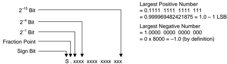
**Figure 39. 2s-Complement Coefficient Format**
