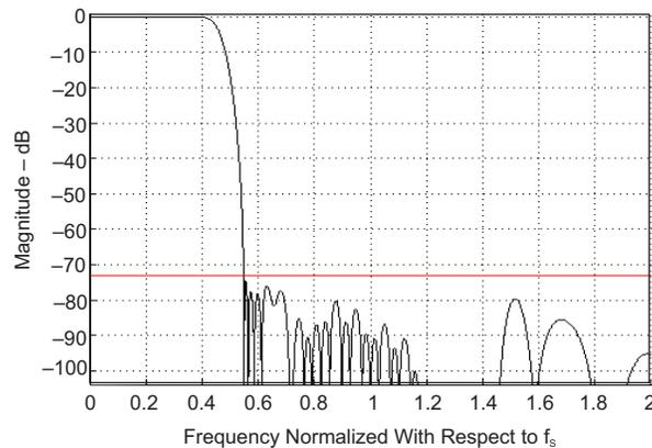
ADC channel response for decimation filter A
