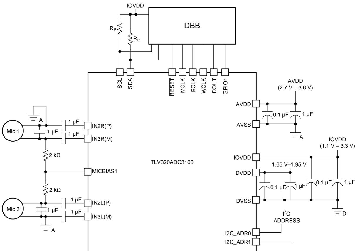
Figure 137. Typical Connections
