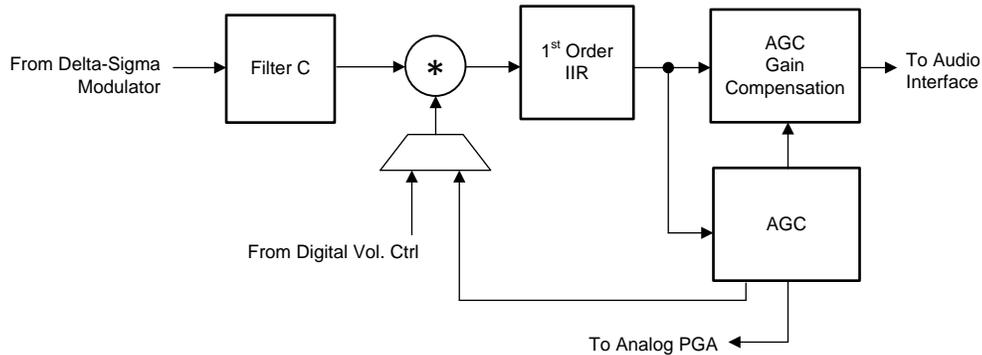
Figure 36. Signal Chain for PRB\_R13 and PRB\_R16
