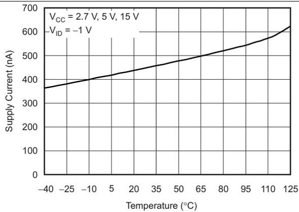
**Figure 7. Supply Current vs Free-Air Temperature**
