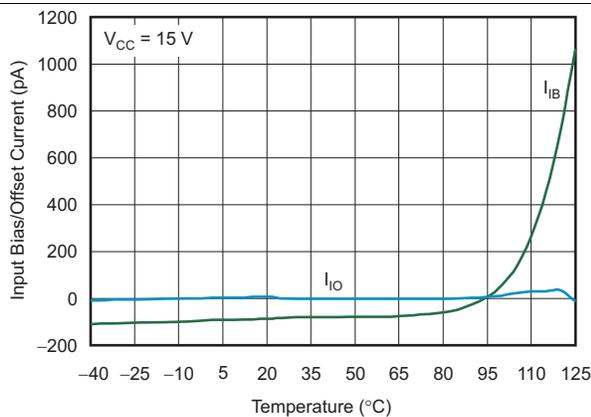
Figure 1. Input Bias/Offset Current vs Free-Air Temperature
