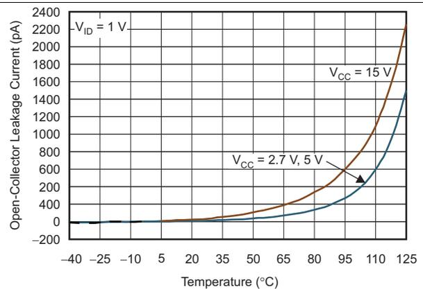
Figure 2. Open-Collector Leakage Current vs Free-Air Temperature
