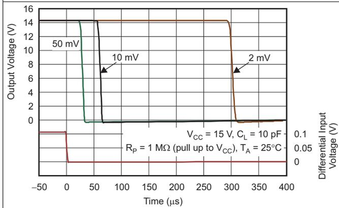
Figure 13. High-to-Low Level Output Response for Various Input Overdrives
