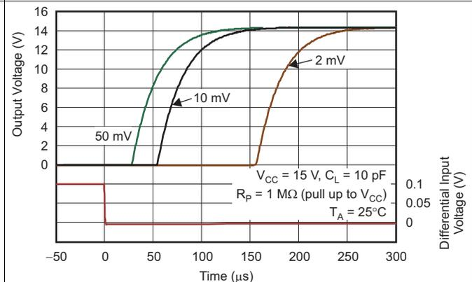
**Figure 10. Low-to-High Level Output Response for Various Input Overdrives**
