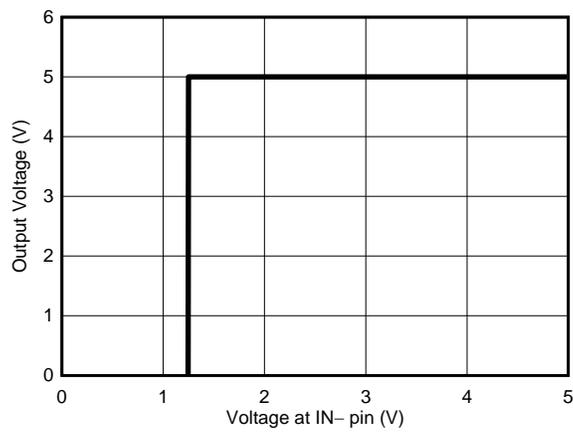
**Figure 17. Transfer Function for the Threshold Detector**
