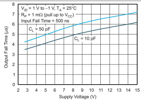
Figure 14. Output Fall Time vs Supply Voltage
