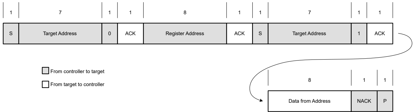
Figure 7-13. Single-byte Read
