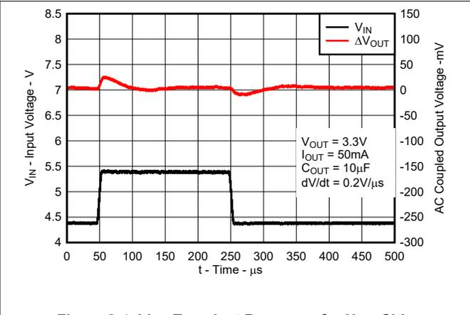
**Figure 8-4. Line Transient Response for New Chip**
