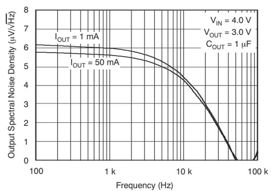
Figure 6-18. Output Spectral Noise Density vs Frequency for Legacy Chip
