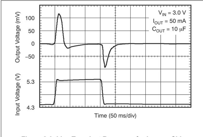
**Figure 8-3. Line Transient Response for Legacy Chip**
