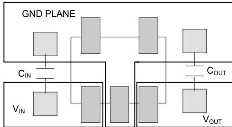
**Figure 8-8. Layout Example for the DBV Package**
