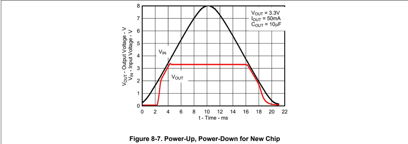
**Figure 8-7. Power-Up, Power-Down for New Chip**
