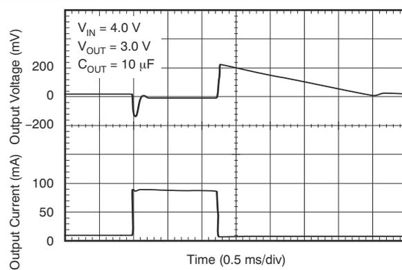
**Figure 6-24. Load Transient Response for Legacy Chip**
