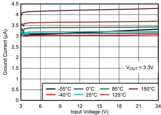
Figure 6-15. Ground Pin Current vs Input Voltage for New Chip
