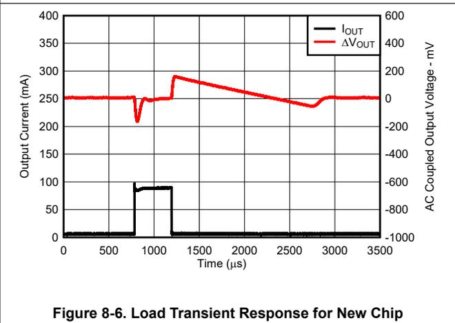
Figure 8-6. Load Transient Response for New Chip
