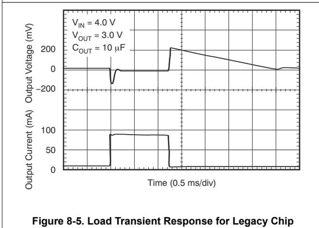
Figure 8-5. Load Transient Response for Legacy Chip
