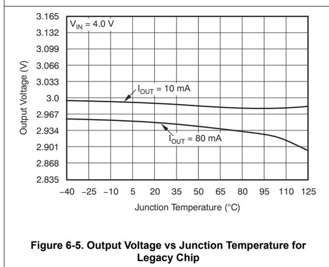
Figure 6-5. Output Voltage vs Junction Temperature for Legacy Chip
