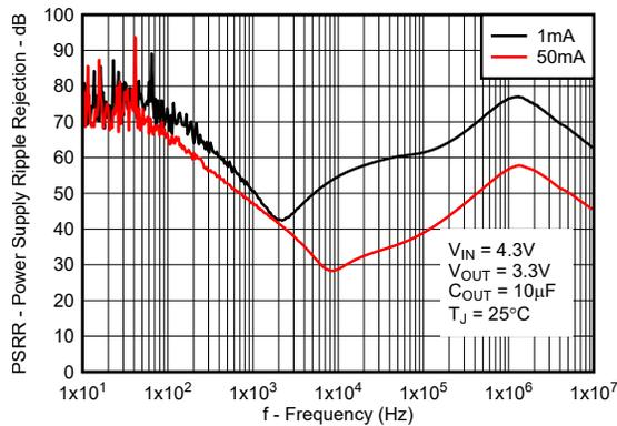
**Figure 6-21. Power-Supply Ripple Rejection vs Frequency for New Chip**
