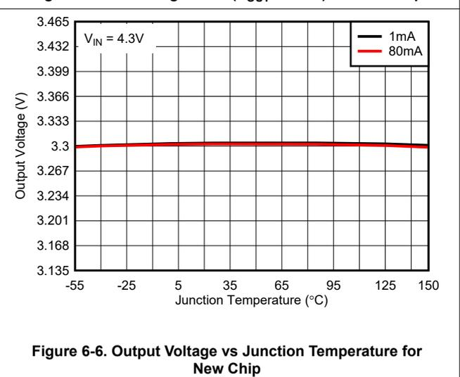
Figure 6-6. Output Voltage vs Junction Temperature for New Chip
