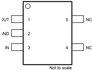
**Figure 5-1. DBV Package, 5-Pin SOT-23 (Top View)**
