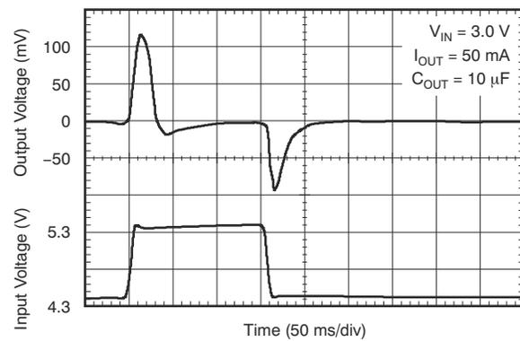
**Figure 6-22. Line Transient Response for Legacy Chip**
