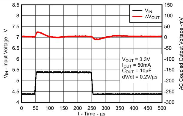
**Figure 6-23. Line Transient Response for New Chip**
