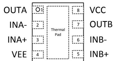
(1) Connect thermal pad to V-.
