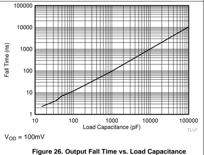
Figure 26. Output Fall Time vs. Load Capacitance
