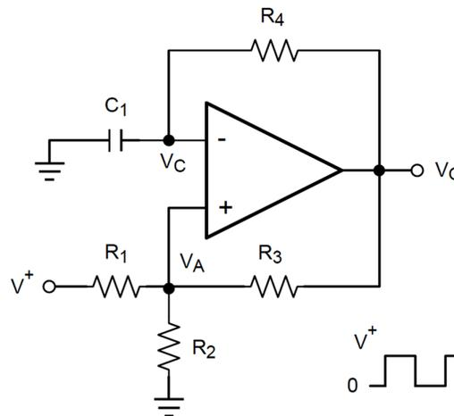
**Figure 39. Square-Wave Oscillator**
