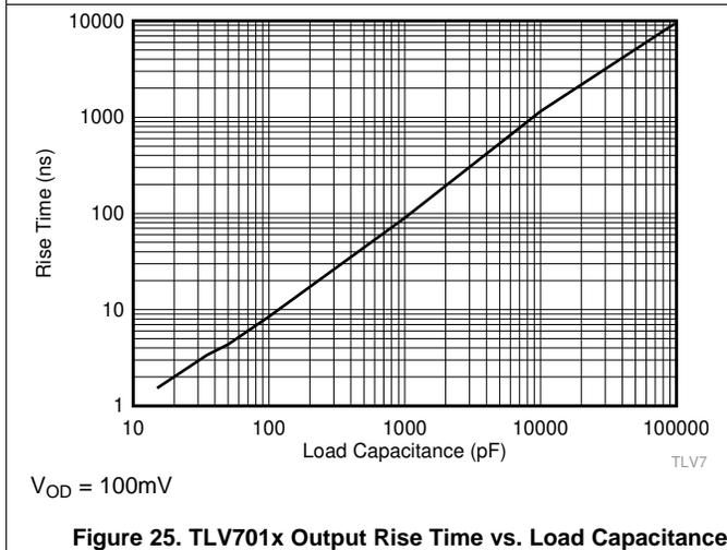
Figure 25. TLV701x Output Rise Time vs. Load Capacitance
