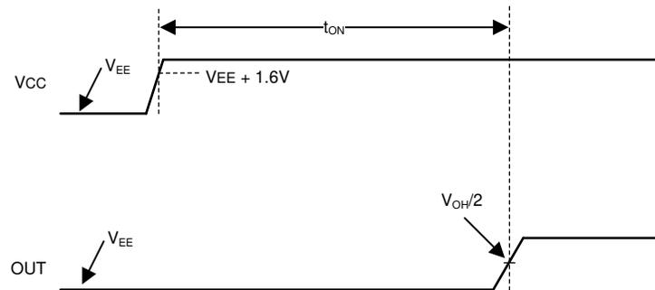
Figure 1. Start-Up Time Timing Diagram (IN+ > IN-)
