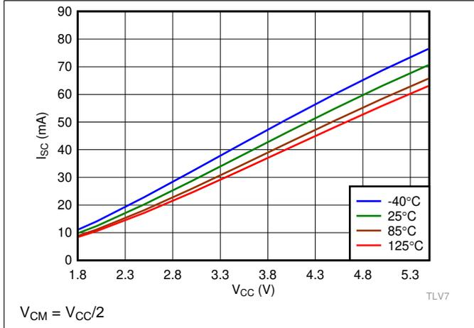
Figure 21. TLV701x Output Short Circuit (Source) vs.  $V_{CC}$
