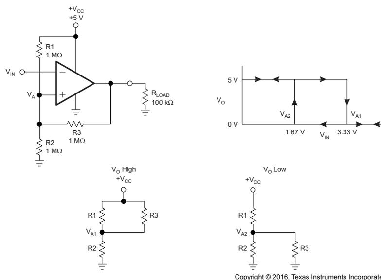
Figure 33. TLV701x in an Inverting Configuration With Hysteresis
