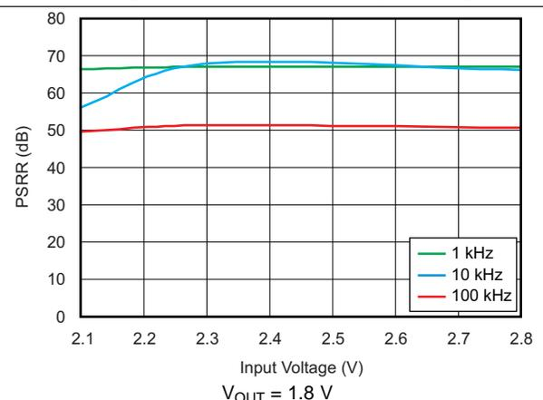
Figure 12. Power-Supply Ripple Rejection vs Input Voltage
