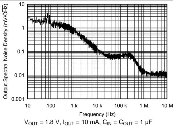
Figure 13. Output Spectral Noise Density vs Frequency
