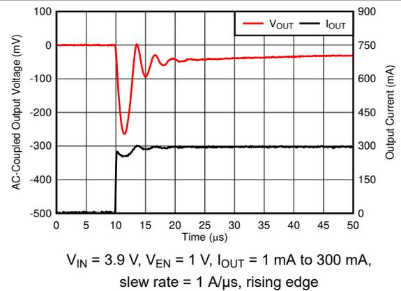
Figure 5-24. Load Transient
