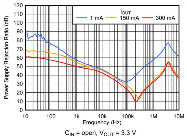
Figure 5-16. PSRR vs Frequency and  $I_{OUT}$
