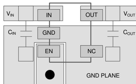
● Represents via used for application-specific connections
