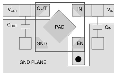
● Represents via used for application-specific connections
