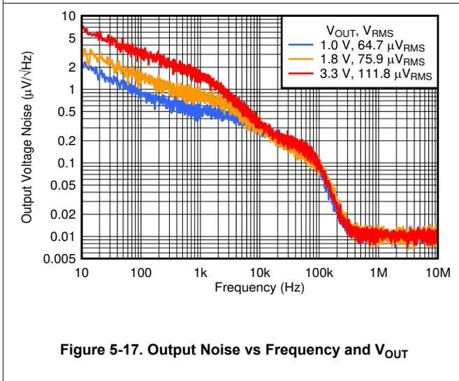
Figure 5-17. Output Noise vs Frequency and  $V_{OUT}$
