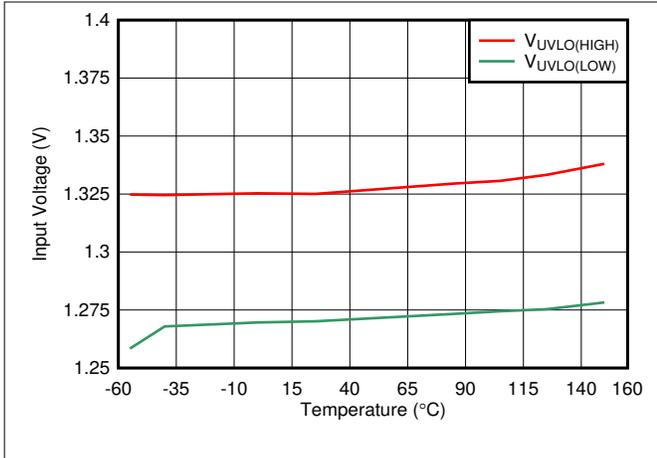
Figure 5-13. UVLO Rising and Falling Threshold vs Temperature
