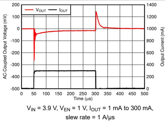
Figure 5-23. Load Transient
