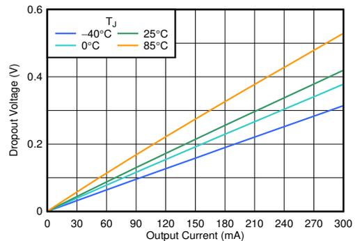
Dropout Voltage vs Output Current (3.3V<sub>OUT</sub>)
