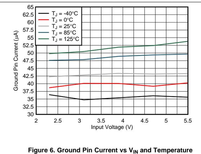
Figure 6. Ground Pin Current vs  $V_{IN}$  and Temperature
