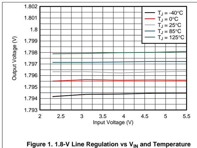
Figure 1. 1.8-V Line Regulation vs  $V_{IN}$  and Temperature
