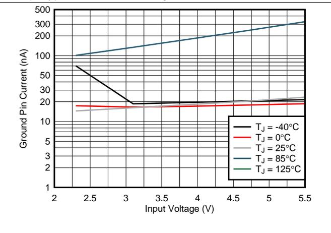
Figure 8. Shutdown Current vs  $V_{IN}$  and Temperature
