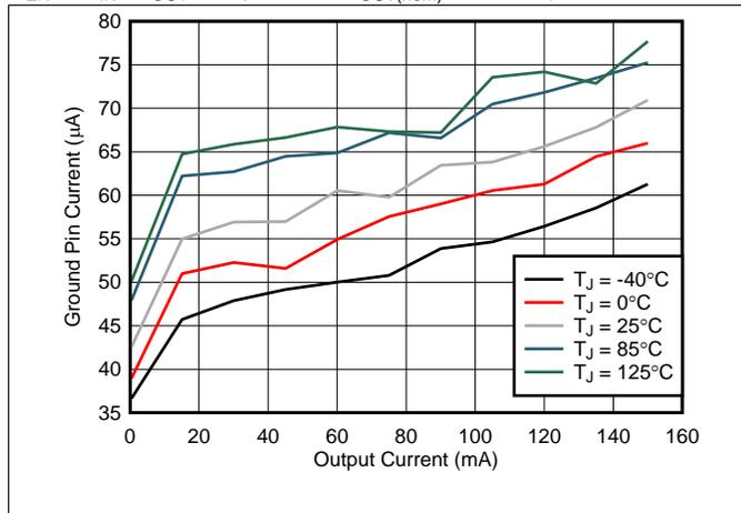
Figure 7. Ground Pin Current vs  $I_{OUT}$  and Temperature
