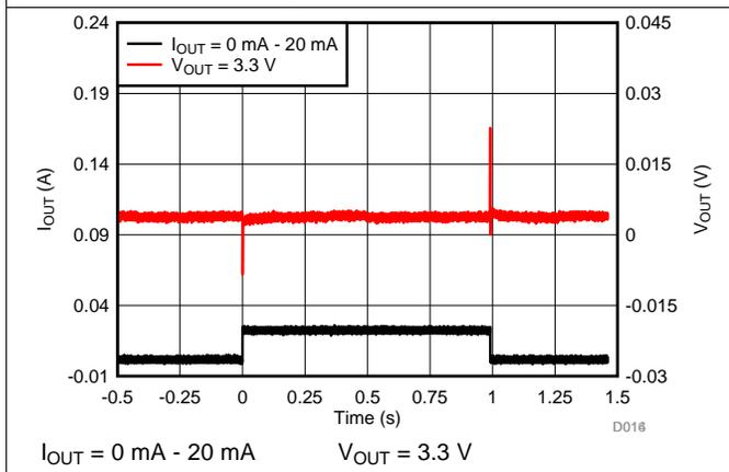
Figure 15. Load Transient
