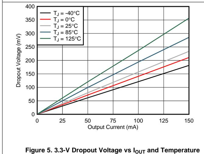
Figure 5. 3.3-V Dropout Voltage vs  $I_{OUT}$  and Temperature
