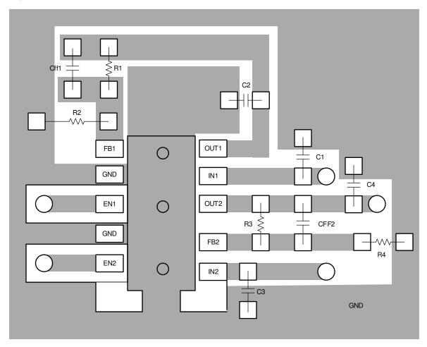
Figure 44. DSQ Package Layout Example
