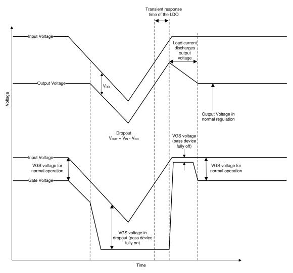
Figure 40. Line Transients From Dropout
