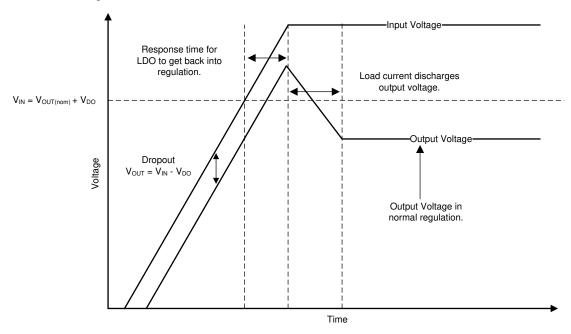
Figure 39. Startup Into Dropout
