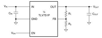
Figure 38. Adjustable Operation
