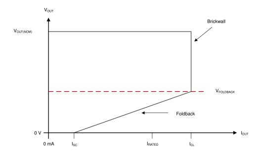
Figure 37. Foldback Current Limit
