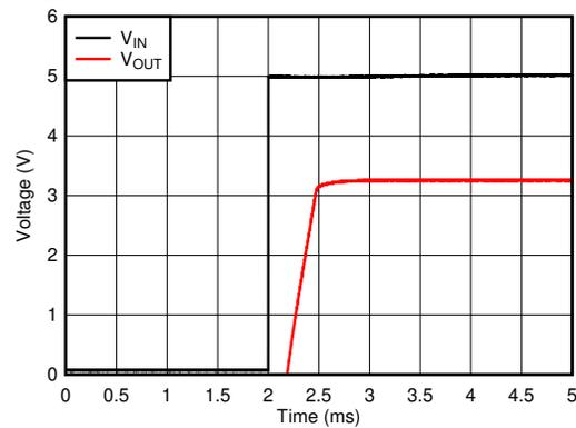
**Figure 5-10.  $V_{IN} = V_{EN}$  Power-Up**
