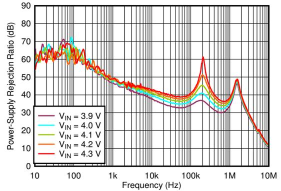
$V_{OUT} = 3.3\text{ V}$ ,  $I_{OUT} = 500\text{ mA}$ ,  $C_{OUT} = 2.2\ \mu\text{F}$
