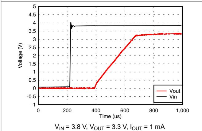
**Figure 5-23.  $V_{IN}$  Power-Up**
