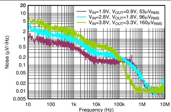
$I_{OUT} = 500\text{ mA}$ ,  $C_{OUT} = 2.2\ \mu\text{F}$ ,  $V_{RMS}\text{ BW} = 10\text{ Hz to }100\text{ kHz}$
