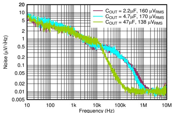
$V_{IN} = 3.8\text{ V}$ ,  $V_{OUT} = 3.3\text{ V}$ ,  $I_{OUT} = 100\text{ mA}$ ,  $C_{FF} = 0\ \mu\text{F}$ ,  $V_{RMS}$  BW = 10 Hz to 100 kHz
