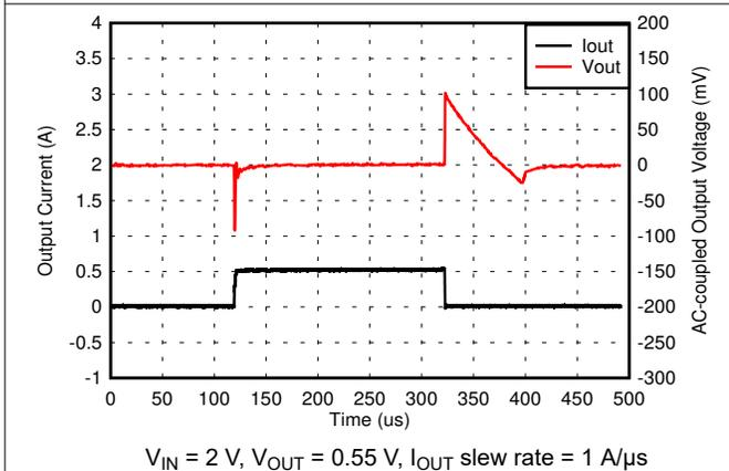
**Figure 5-21. 0.55-V, 1-mA to 500-mA Load Transient**
