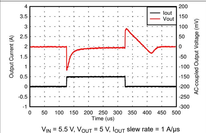
**Figure 5-22. 5-V, 1-mA to 500-mA Load Transient**
