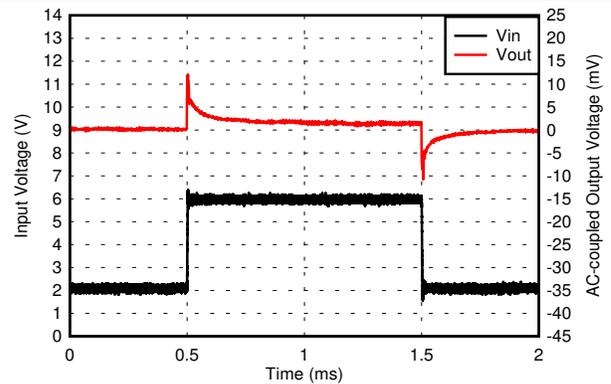
$V_{OUT} = 0.55\text{ V}$ ,  $I_{OUT} = 1\text{ mA}$ ,  $V_{IN}$  slew rate =  $1\text{ V}/\mu\text{s}$
