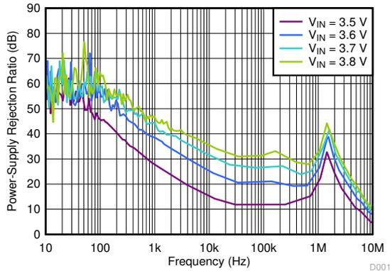
$V_{OUT} = 3.3\text{ V}$ ,  $I_{OUT} = 500\text{ mA}$ ,  $C_{OUT} = 2.2\ \mu\text{F}$
