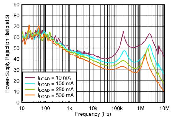
$V_{IN} = 3.8\text{ V}$ ,  $V_{OUT} = 3.3\text{ V}$ ,  $C_{OUT} = 2.2\ \mu\text{F}$
