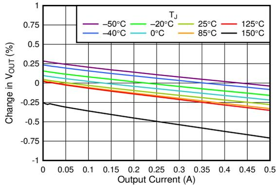
$V_{IN} = 6\text{ V}$ ,  $V_{OUT} = 5.5\text{ V}$
