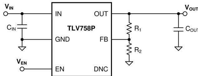
Figure 7-1. Adjustable Operation
