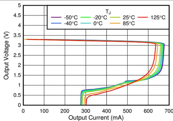
Figure 5-17. 3.3-V Foldback Current Limit vs  $I_{OUT}$
