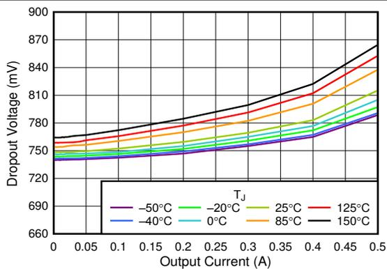
Figure 5-5. 0.55-V Dropout Voltage vs  $I_{OUT}$
