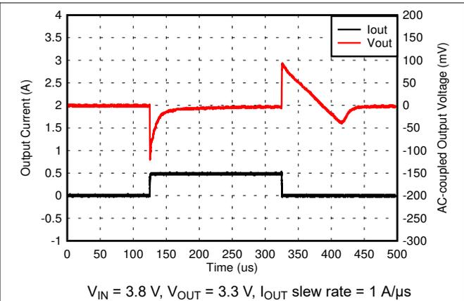
**Figure 5-20. 3.3-V, 1-mA to 500-mA Load Transient**
