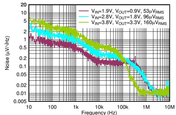
$I_{OUT} = 500\text{ mA}$ ,  $C_{OUT} = 2.2\ \mu\text{F}$ ,  $V_{RMS}$  BW = 10 Hz to 100 kHz
