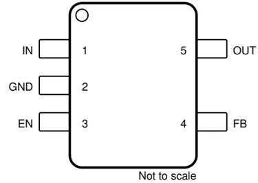
**Figure 4-1. DRV Package, 6-Pin Adjustable WSON (Top View)**
