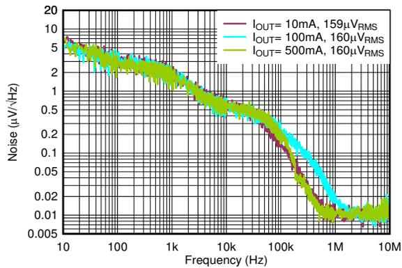
$V_{IN} = 3.8\text{ V}$ ,  $V_{OUT} = 3.3\text{ V}$ ,  $C_{OUT} = 2.2\ \mu\text{F}$ ,  $V_{RMS}$  BW = 10 Hz to 100 kHz
