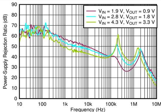
$I_{OUT} = 500\text{ mA}$ ,  $C_{OUT} = 2.2\ \mu\text{F}$
