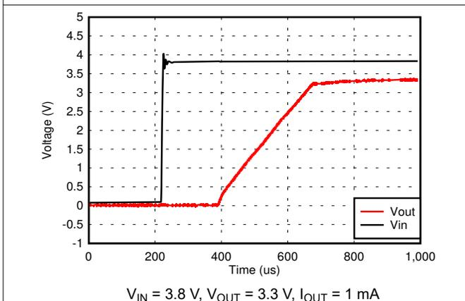
**Figure 5-23.  $V_{IN}$  Power-Up**
