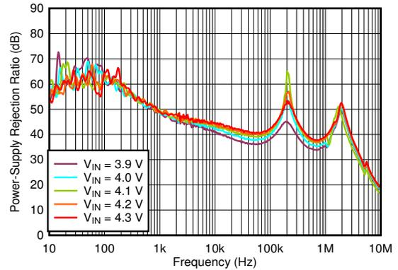
$V_{OUT} = 3.3\text{ V}$ ,  $I_{OUT} = 250\text{ mA}$ ,  $C_{OUT} = 2.2\ \mu\text{F}$
