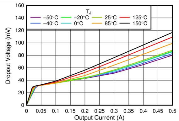
Figure 5-6. 5.5-V Dropout Voltage vs  $I_{OUT}$
