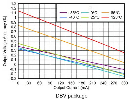
Figure 5-4. Output Voltage Accuracy vs  $I_{OUT}$
