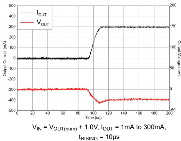
Figure 5-11. Load Transient
