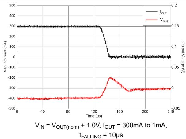
Figure 5-12. Load Transient
