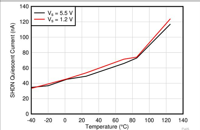
**Figure 6-42. Shutdown Mode Quiescent Current vs Temperature**
