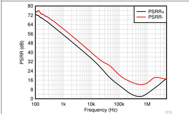
**Figure 6-17. PSRR vs Frequency**
