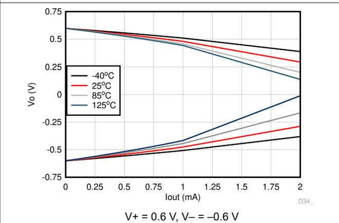
**Figure 6-16. Output Voltage vs Output Current (Claw)**
