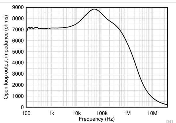
Figure 6-12. Open-Loop Output Impedance vs Frequency
