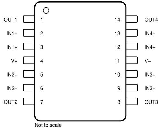
**Figure 5-9. TLV9044 D, PW and DYY Packages
