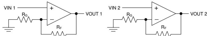
**Figure 8-3. Schematic Representation**
