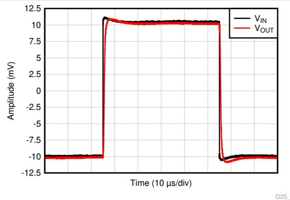
$G = 1$   $V_{IN} = 20\text{ mV}_{PP}$   $C_L = 10\text{ pF}$
