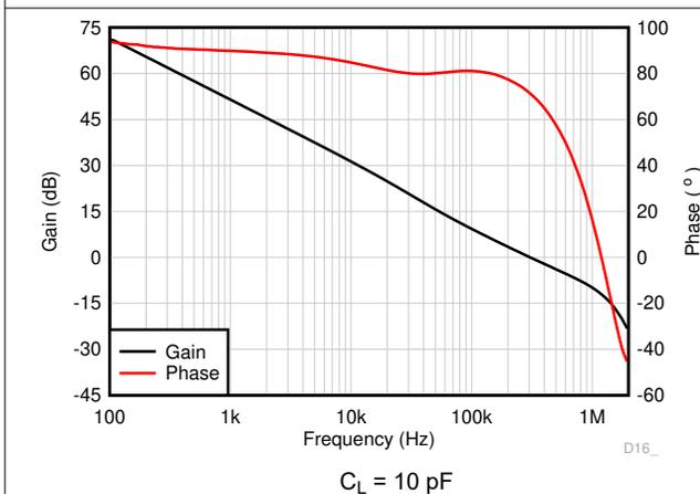
Figure 6-11. Open-Loop Gain and Phase vs Frequency
