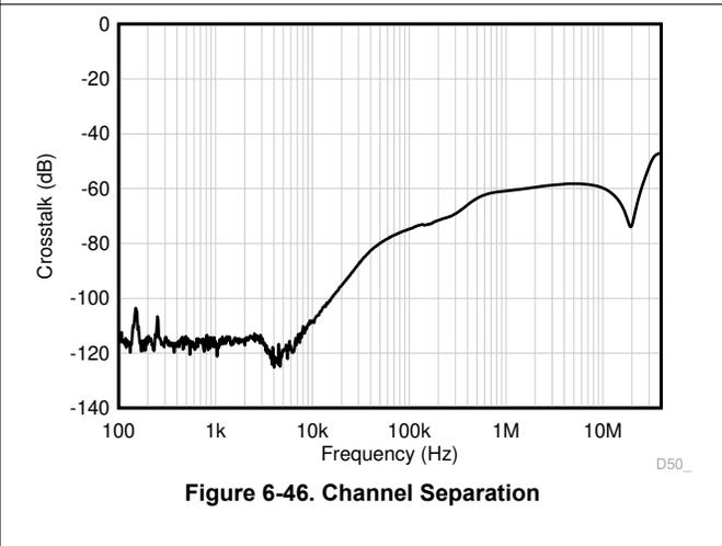
**Figure 6-46. Channel Separation**
