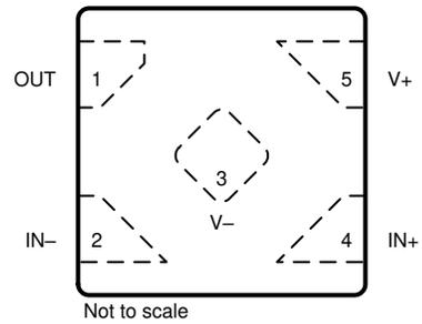
**Figure 5-4. TLV9041 DPW Package 5-Pin X2SON Top View**
