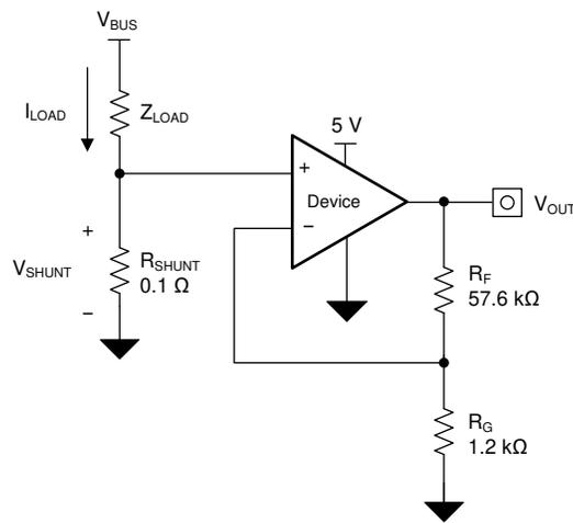
**Figure 8-1. TLV904x in a Low-Side, Current-Sensing Application**
