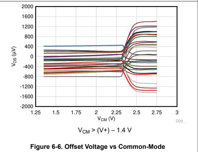
**Figure 6-6. Offset Voltage vs Common-Mode**
