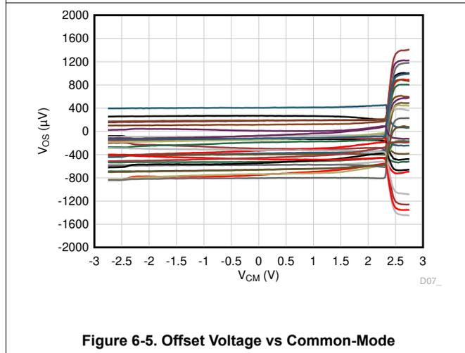
**Figure 6-5. Offset Voltage vs Common-Mode**
