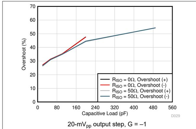
Figure 5-31. Small-Signal Overshoot vs Capacitive Load
