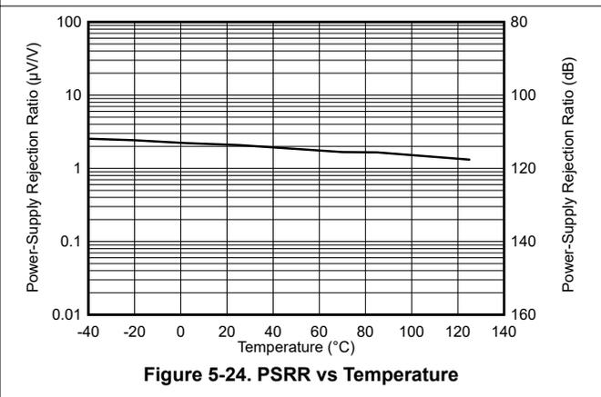
**Figure 5-24. PSRR vs Temperature**
