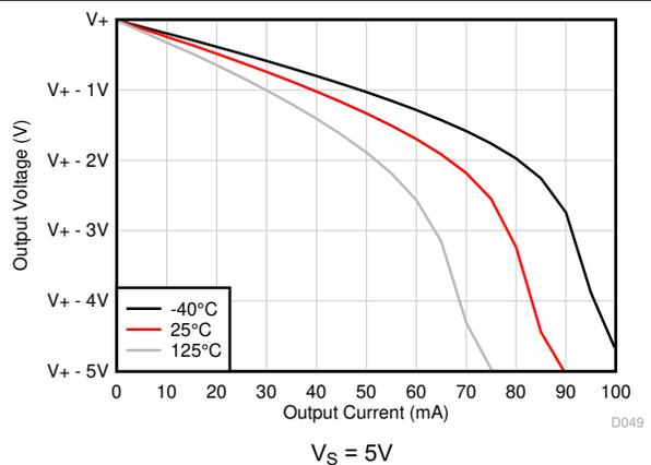
**Figure 5-18. Output Voltage Swing vs Output Current (Sourcing)**
