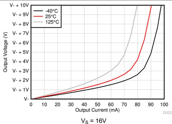
**Figure 5-17. Output Voltage Swing vs Output Current (Sinking)**
