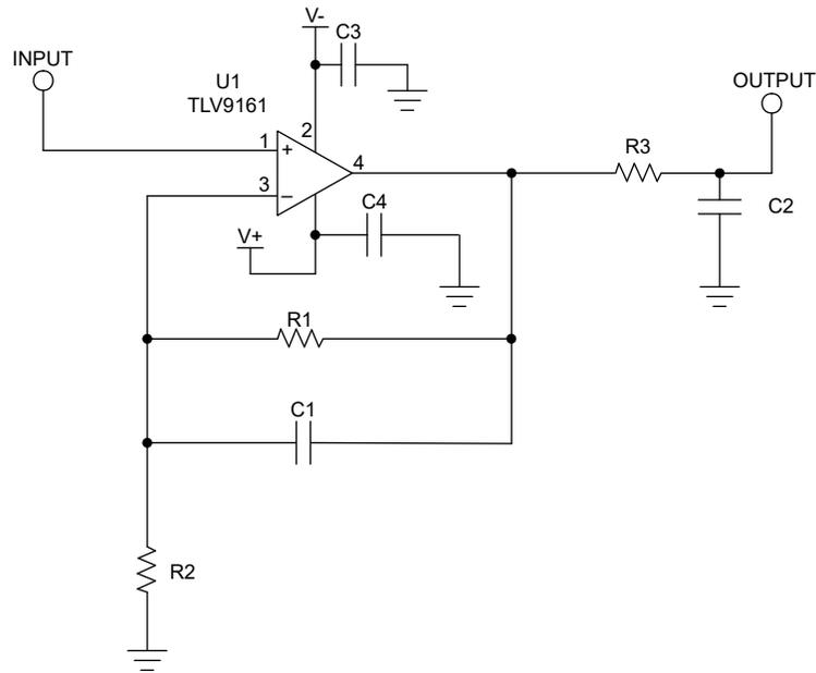
Figure 7-4. Schematic for Noninverting Configuration Layout Example
