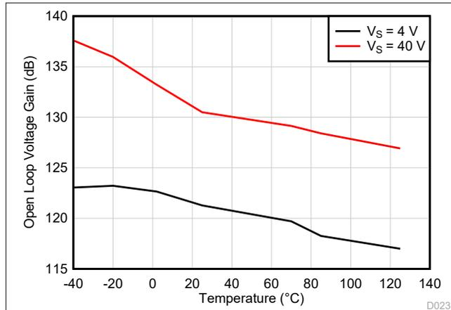
Figure 5-25. Open-Loop Voltage Gain vs Temperature (dB)
