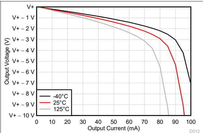
Figure 5-14. Output Voltage Swing vs Output Current (Sourcing)
