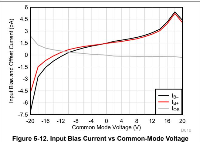
**Figure 5-12. Input Bias Current vs Common-Mode Voltage**
