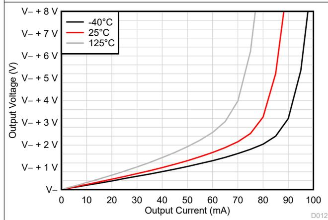
Figure 5-15. Output Voltage Swing vs Output Current (Sinking)
