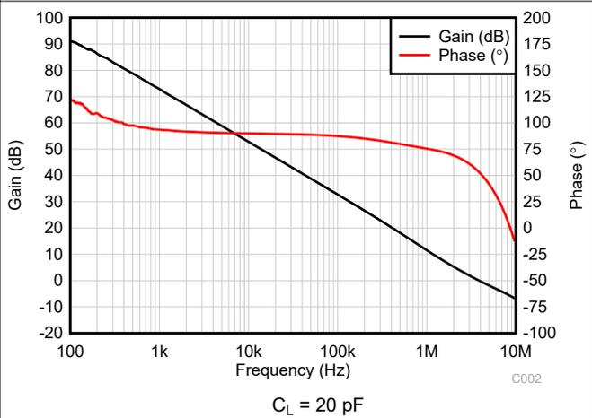
**Figure 5-10. Open-Loop Gain and Phase vs Frequency**
