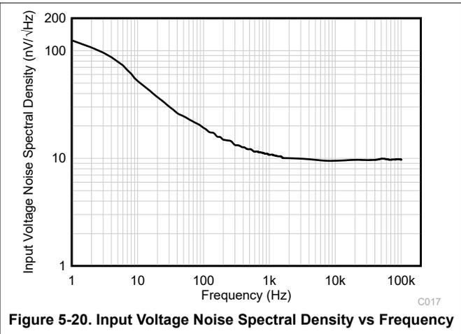
**Figure 5-20. Input Voltage Noise Spectral Density vs Frequency**
