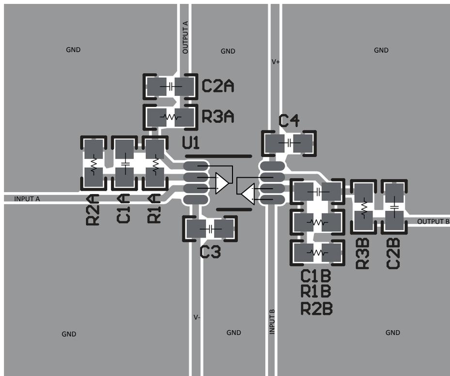
**Figure 7-6. Example Layout for VSSOP-8 (DGK) Package**
