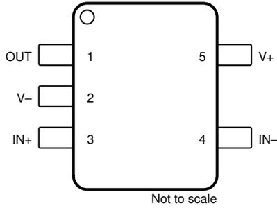
**Figure 4-1. TLV9351-Q1 DBV Package,
