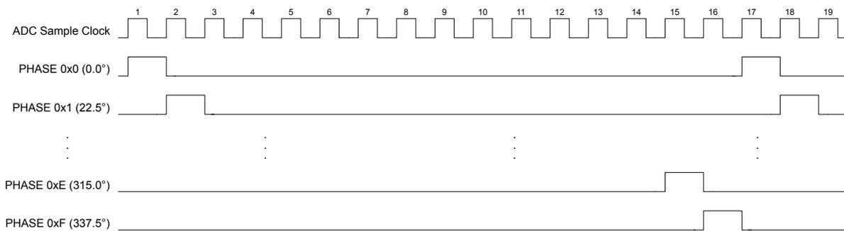
This feature can be used to double the sampling rate of an input. Both ADC module 0 and ADC module 1 can be programmed to sample the same input. ADC module 0 could sample at the standard position (the  $PHASE$  field in the **ADCSPC** register is 0x0). ADC module 1 can be configured to sample at 180 ( $PHASE = 0x8$ ). The two modules can be synchronized using the  $GSYNC$  and  $SYNCWAIT$
