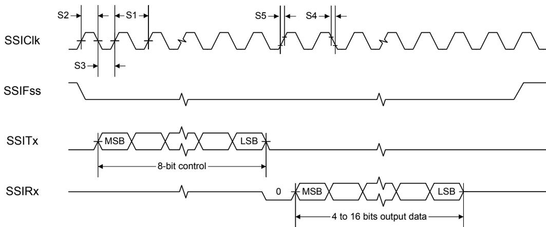
Figure 22-21. Master Mode SSI Timing for SPI Frame Format (FRF=00), with SPH=1
