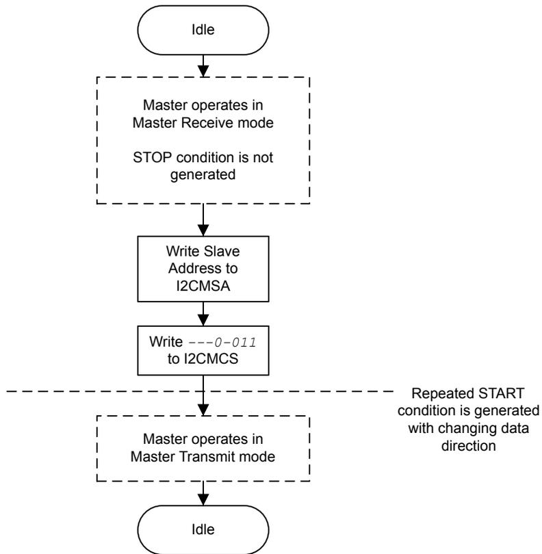
Figure 16-14. Standard High Speed Mode Master Transmit
