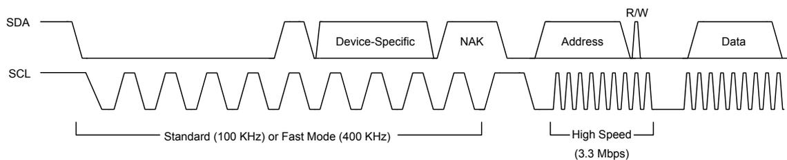
**Note:** High-Speed mode is 3.4 Mbps, provided correct system clock frequency is set and there is appropriate pull strength on SCL and SDA lines.
