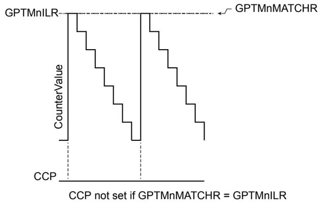
Figure 11-8 on page 692 shows how the CCP output operates when the `PLO` and `MRSU` bits are set and the `GPTMTnILR` is greater than the `GPTMTnMATCHR` value.
