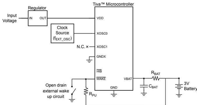
**Note:** Some devices may not supply the GNDX,  $\overline{\text{WAKE}}$  or  $\overline{\text{HIB}}$  signals. See “Signal Tables” on page 1141 for pins specific to your device.
