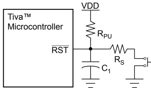
Typical  $R_{PU} = 10\text{ k}\Omega$
