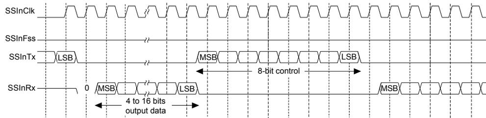
In the MICROWIRE mode, the SSI slave samples the first bit of receive data on the rising edge of  $SSInClk$  after  $SSInFss$  has gone Low. Masters that drive a free-running  $SSInClk$  must ensure that the  $SSInFss$  signal has sufficient setup and hold margins with respect to the rising edge of  $SSInClk$ .
