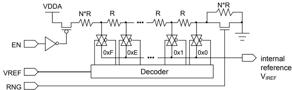
**Note:** In the figure above,  $N \cdot R$  represents a multiple of the  $R$  value that produces the results specified in Table 19-2 on page 1128.
