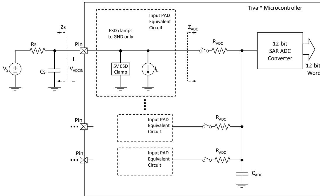
The ADC operates from both the 3.3-V analog and 1.2-V digital power supplies. The ADC clock can be configured to reduce power consumption when ADC conversions are not required (see “System Control” on page 219). The analog inputs are connected to the ADC through specially balanced input paths to minimize the distortion and cross-talk on the inputs. Detailed information on the ADC power supplies and analog inputs can be found in “Analog-to-Digital Converter (ADC)” on page 1194.
