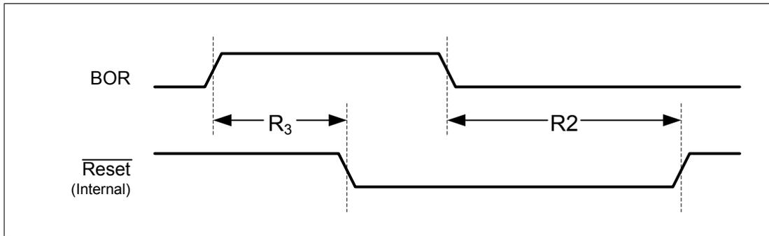
Figure 22-11. External Reset Timing ( $\overline{\text{RST}}$ )
