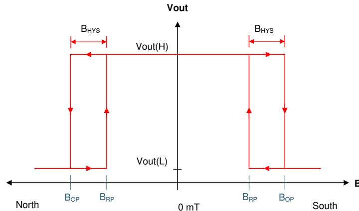
**Figure 8-3. Omnipolar Functionality**
