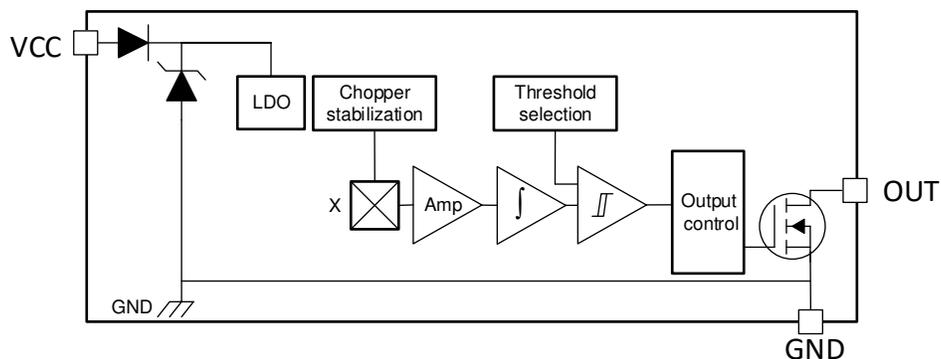
Figure 8-1. Block Diagram
