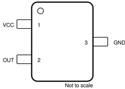
**Figure 6-1. DBZ Package 3-Pin SOT-23 Top View**
