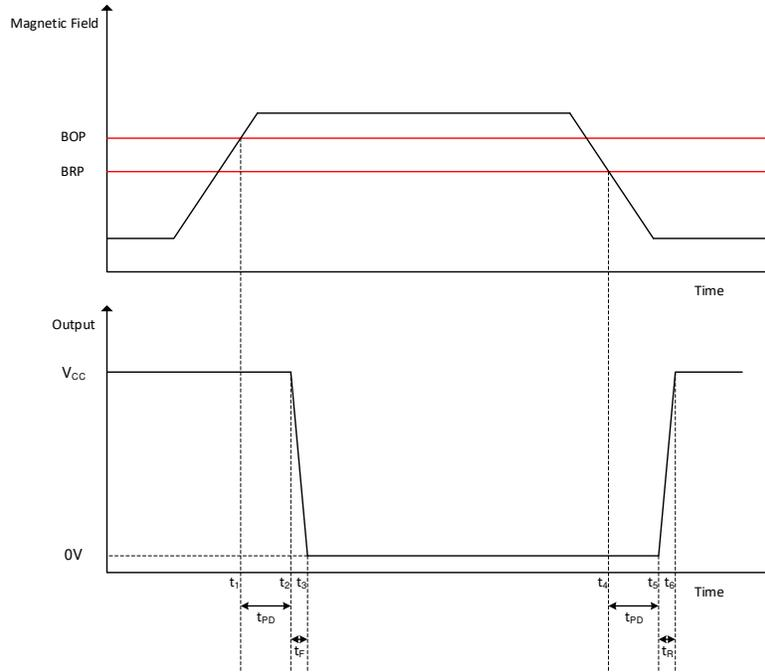
**Figure 8-8. Propagation Delay**
