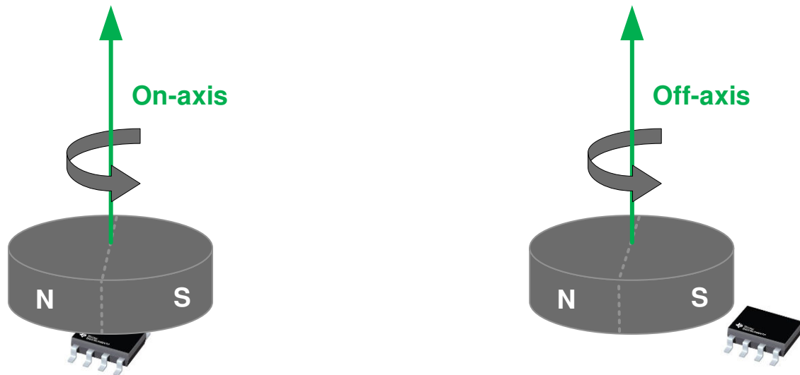
Figure 8-5. On-Axis vs. Off-Axis Angle Measurements
