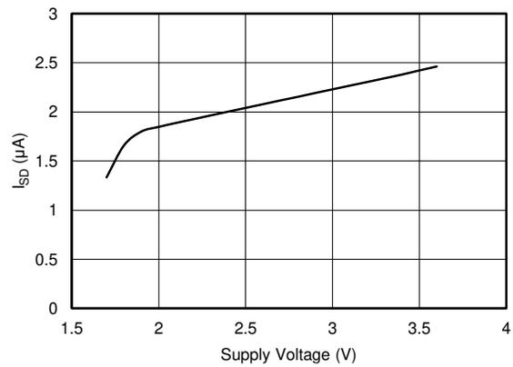
Figure 6-11. Shutdown Quiescent Current vs. Supply Voltage
