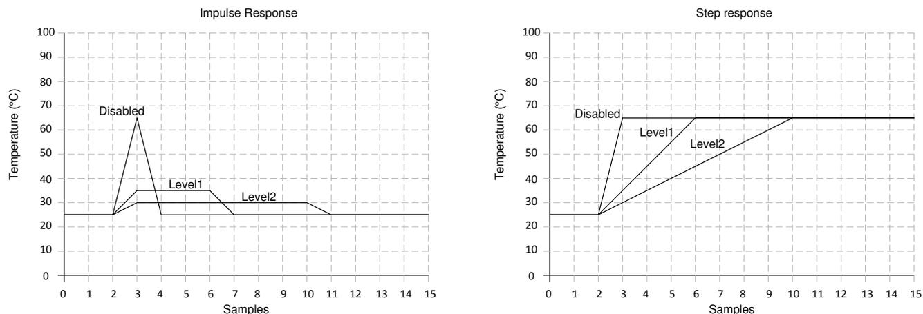
**Figure 7-1. Filter Response to Impulse and Step Inputs**
