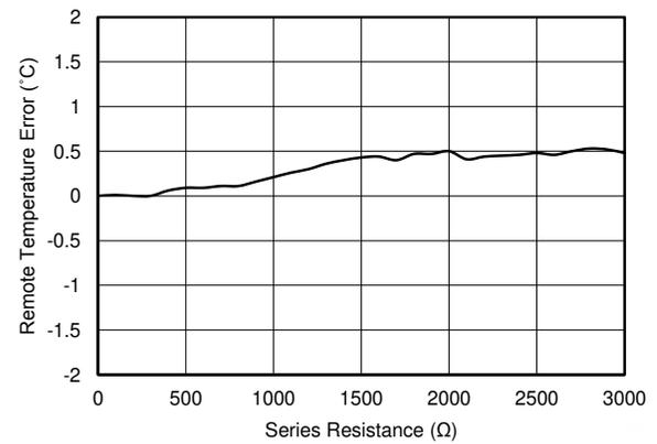
**Figure 6-5. Remote Temperature Error vs. Series Resistance**
