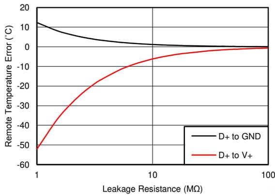
**Figure 6-4. Remote Temperature Error vs. Leakage Resistance**
