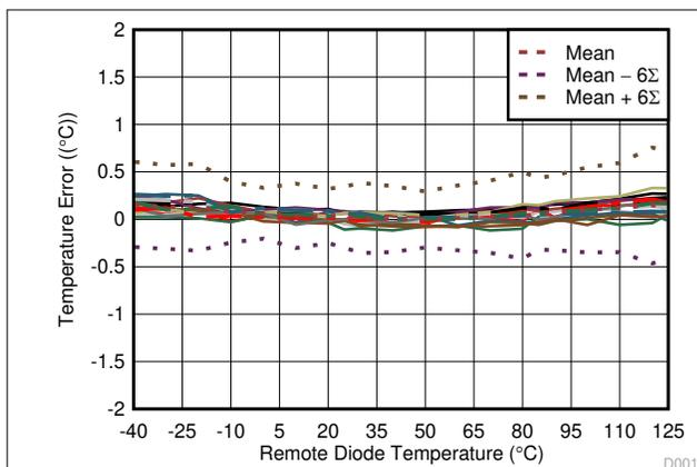
**Figure 8-3. TMP451-Q1 Remote Diode Temperature Drift (Diode-Connected 2N3906)**
