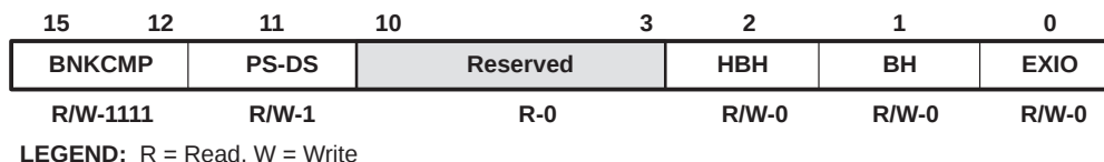
Figure 6. Bank-Switching Control Register (BSCR), MMR Address 0029h
