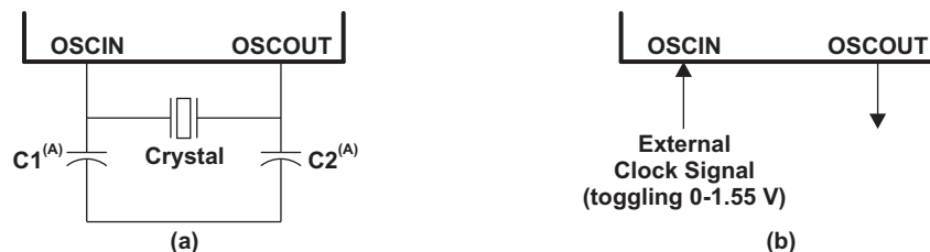
Figure 5-3. Recommended Crystal/Clock Connection
