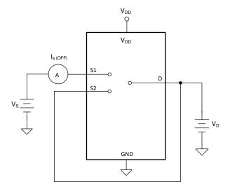
Figure 6-2. Off-Leakage Measurement Setup
