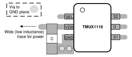
Figure 8-4. TMUX1119 Layout Example
