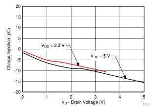
Figure 7-4. Charge Injection vs Drain Voltage
