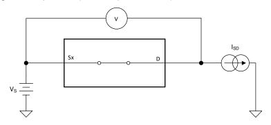
Figure 6-1. On-Resistance Measurement Setup
