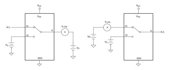
Figure 6-3. On-Leakage Measurement Setup
