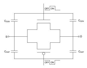
Figure 7-3. Transmission Gate Topology
