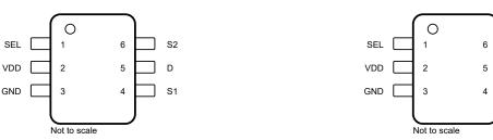
Figure 4-1. DCK Package, 6-Pin SC70 (Top View) Figure 4-2. DBV Package, 6-Pin SOT-23 (Top View)
