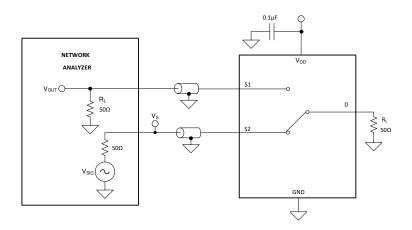
Figure 6-8. Crosstalk Measurement Setup
