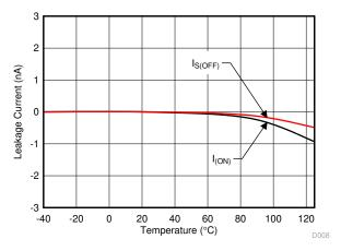
Figure 7-2. Leakage Current vs Temperature
