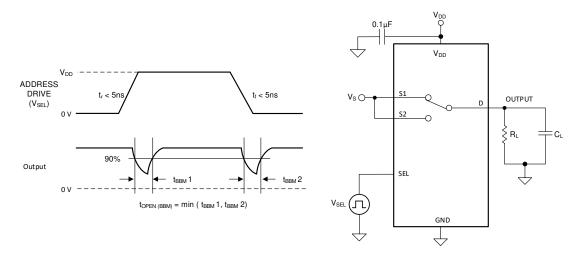
Figure 6-5. Break-Before-Make Delay Measurement Setup
