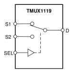
Figure 7-1. TMUX1119 Functional Block Diagram
