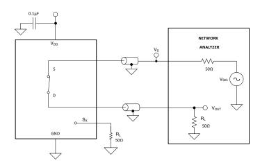
Figure 6-9. Bandwidth Measurement Setup
