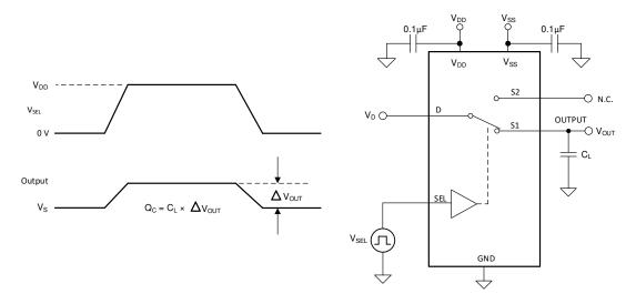
Figure 6-6. Charge-Injection Measurement Setup
