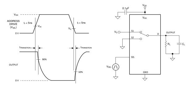
Figure 6-4. Transition-Time Measurement Setup
