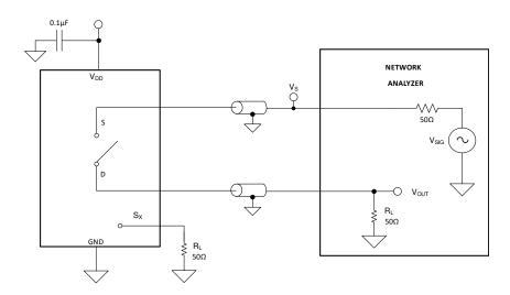
Figure 6-7. Off Isolation Measurement Setup
