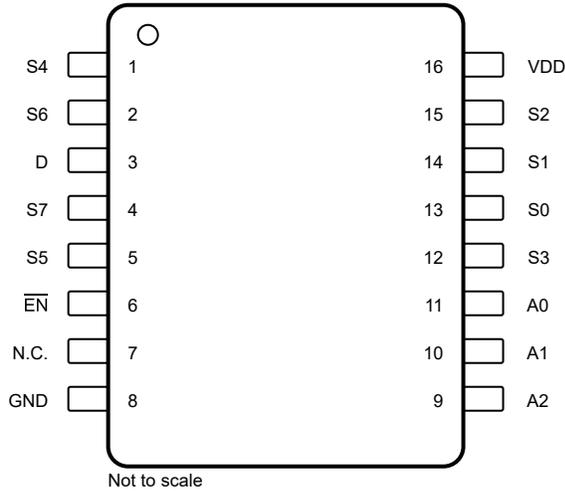
**Figure 5-1. TMUX1308-Q1: PW Package, 16-Pin TSSOP (Top View)**
