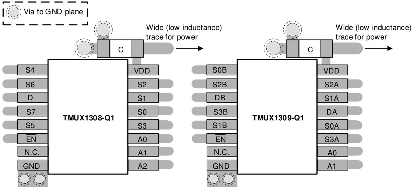
Figure 9-7. TMUX1308-Q1 and TMUX1309-Q1 Layout Example
