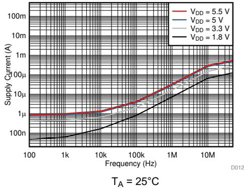
Figure 6-7. Supply Current vs Input Switching Frequency
