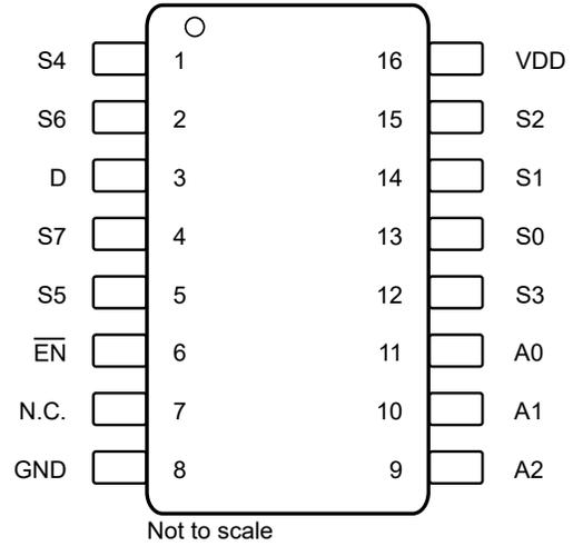
**Figure 5-2. TMUX1308-Q1: DYY Package, 16-Pin SOT-23-THIN (Top View)**
