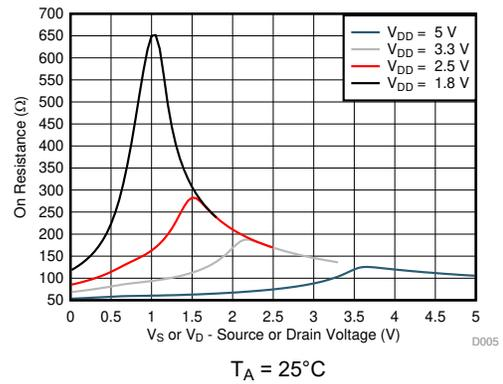
Figure 6-4. On-Resistance vs Source or Drain Voltage
