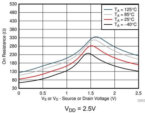
Figure 6-3. On-Resistance vs Temperature
