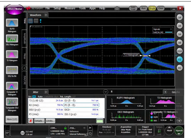
Figure 6-10. Through a Typical TMUXHS221LV Channel at 3Gbps
