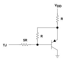
Figure 70. TJ Terminal Internal Circuit
