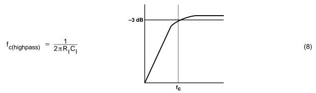
The value of  $C_I$  is important to consider as it directly affects the bass (low frequency) performance of the circuit. Consider the example where  $R_I$  is 10 k $\Omega$  and the specification calls for a flat bass response down to 40 Hz. Equation 8 is reconfigured as equation 9.
