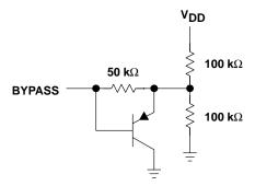
Figure 64. PNP Transistor Clamping of BYPASS Terminal
