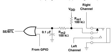
Figure 65. Implementation with an OR Gate
