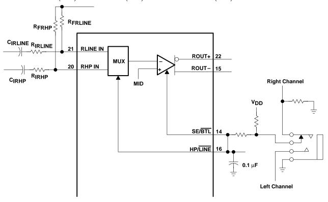
Figure 69. TPA0202 Example Input MUX Circuit
