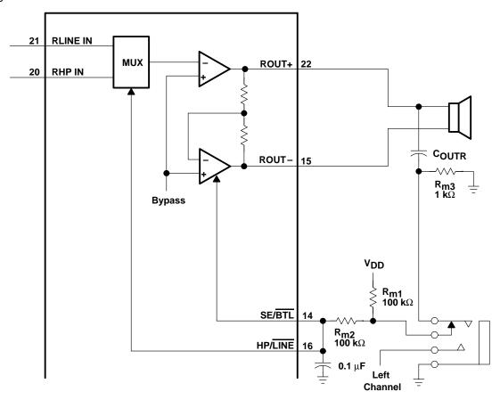
Figure 68. TPA0202 Resistor Divider Network Circuit
