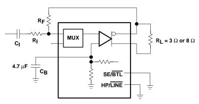
Figure 1. BTL Test Circuit
