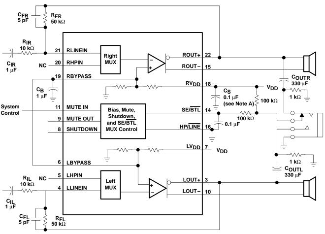
NOTE A: A 0.1 μF ceramic capacitor should be placed as close as possible to the IC. For filtering lower-frequency noise signals, a larger aluminum electrolytic capacitor of 10 μF or greater should be placed near the audio power amplifier.
