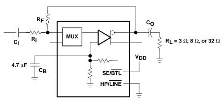
Figure 2. SE Test Circuit
