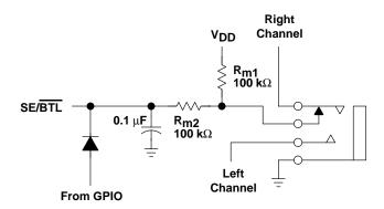
Figure 66. Implementation with a Diode
