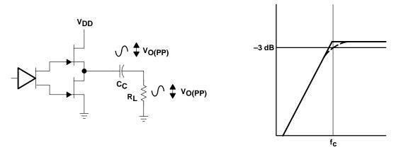
Figure 60. Single-Ended Configuration and Frequency Response
