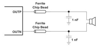
Figure 8-3. Typical Ferrite Chip Bead Filter (Chip Bead Example: NFZ2MSM series from Murata)
