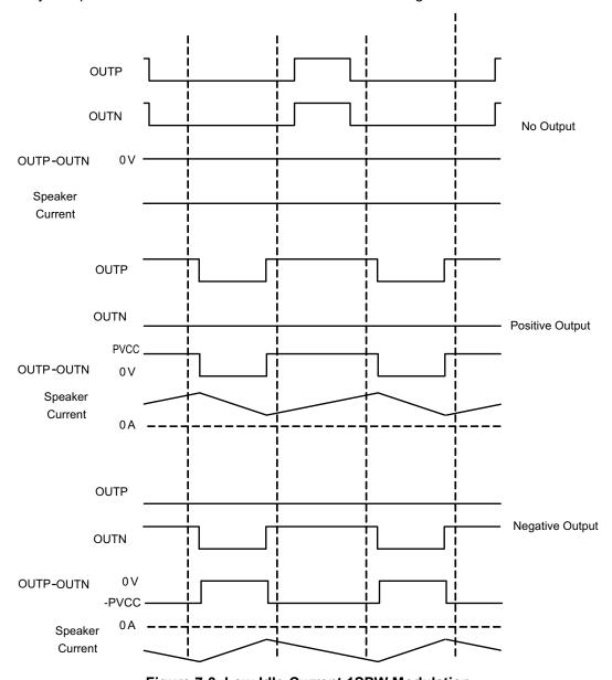
Figure 7-3. Low-Idle-Current 1SPW Modulation
