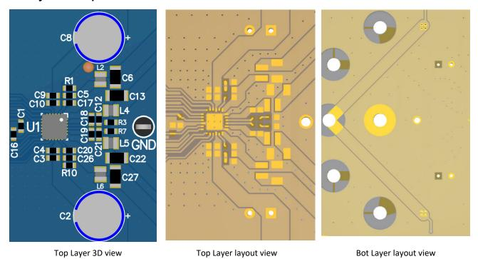
Figure 10-1. BTL Layout Example
