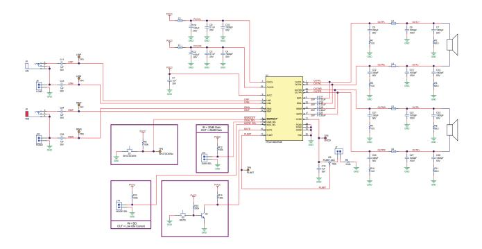
Figure 8-1. Stereo Class-D Amplifier in BTL Configuration with Single-Ended Inputs, Spread Spectrum Modulation and BD Mode
