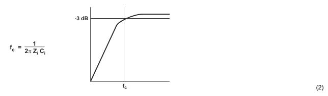
The value of  $C_i$  is important, as it directly affects the bass (low-frequency) performance of the circuit. Consider the example where  $Z_i$  is 20 k $\Omega$  (26dB Gain) and the specification calls for a flat bass response down to 20 Hz. Equation 2 is reconfigured as Equation 3.
