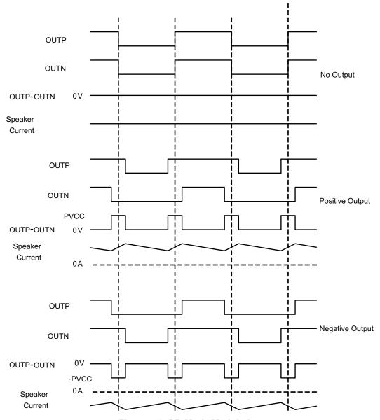
Figure 7-2. BD Mode Modulation
