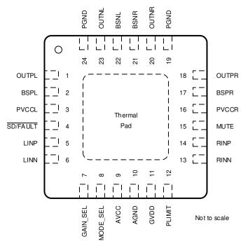
Figure 5-1. RGE Package, 24-Pin VQFN, (Top View)
