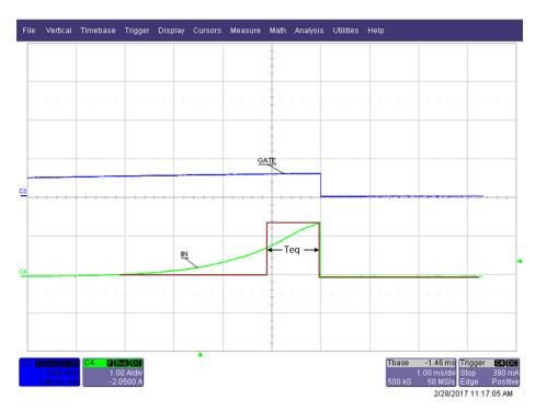
Figure 13. Teq During a Start Into a Short
