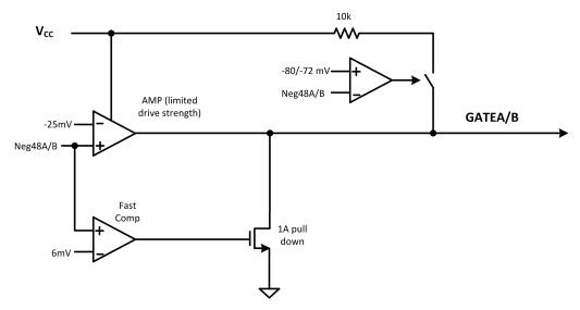
Figure 10. Simplified Diagram of OR-ing Block
