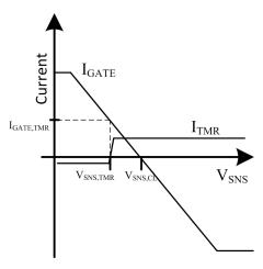
Figure 7. Relationship Between Timer, Gate Current, and Sense Voltage (V<sub>GATE</sub> = 5 V)
