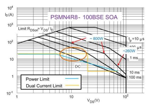
Figure 8. Dual Current Limit vs FET Power Limit
