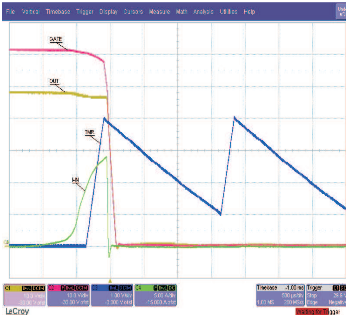
Figure 16. TPS2480/81 Restart Cycle Timing
