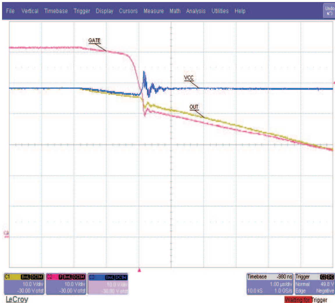
Figure 15. Current Limit Onset
