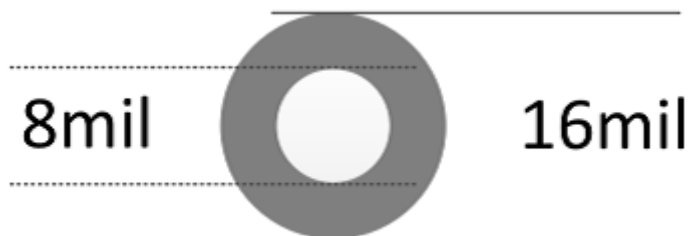
Figure 11-6. Recommended Minimum Via Sizing
