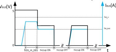
Figure 10-12. BUS Overcurrent Protection
