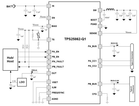
Figure 11-2. TPS25862-Q1 Typical Application Circuit for 2.1-MHz f<sub>sw</sub>
