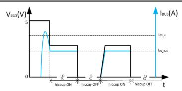
Figure 10-13. BUS Overcurrent Protection: Two-Level Current Limit
