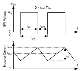
Figure 10-2. SW Node and Inductor Current Waveforms in Continuous Conduction Mode (CCM)
