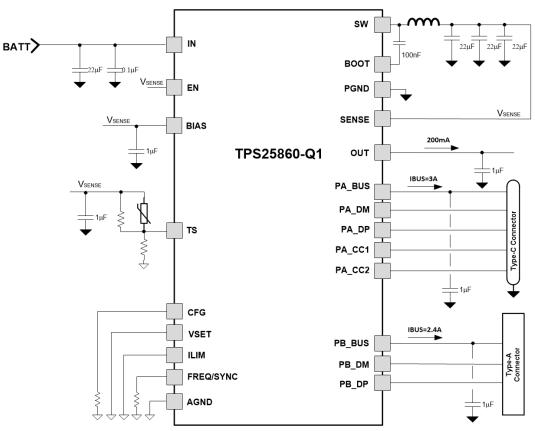
Figure 11-1. TPS25860-Q1 Typical Application Circuit for 2.1-MHz f<sub>SW</sub>
