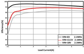
Efficiency vs Output Current
