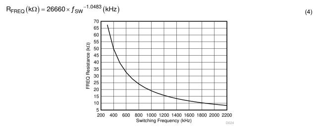
Figure 10-3. FREQ Set Resistor vs Switching Frequency
