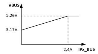
Figure 10-15. Dual Ports Cable Compensation
