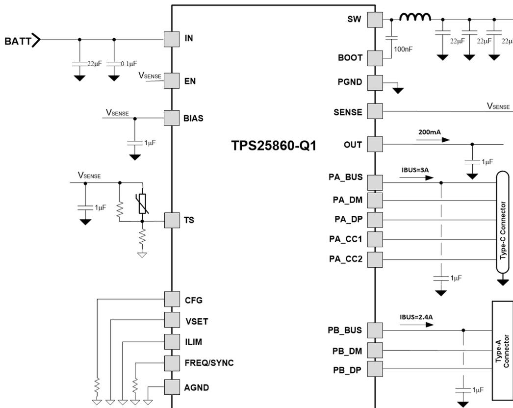
Figure 11-1. TPS25860-Q1 Typical Application Circuit for 2.1-MHz  $f_{SW}$
