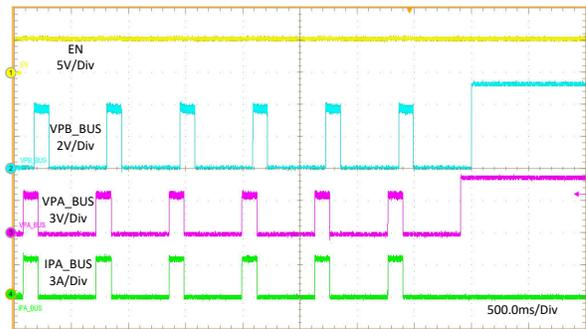
**Figure 11-26. 1-Ω Load Recovery**
