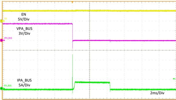
**Figure 11-27. VBUS Hot Short to GND**
