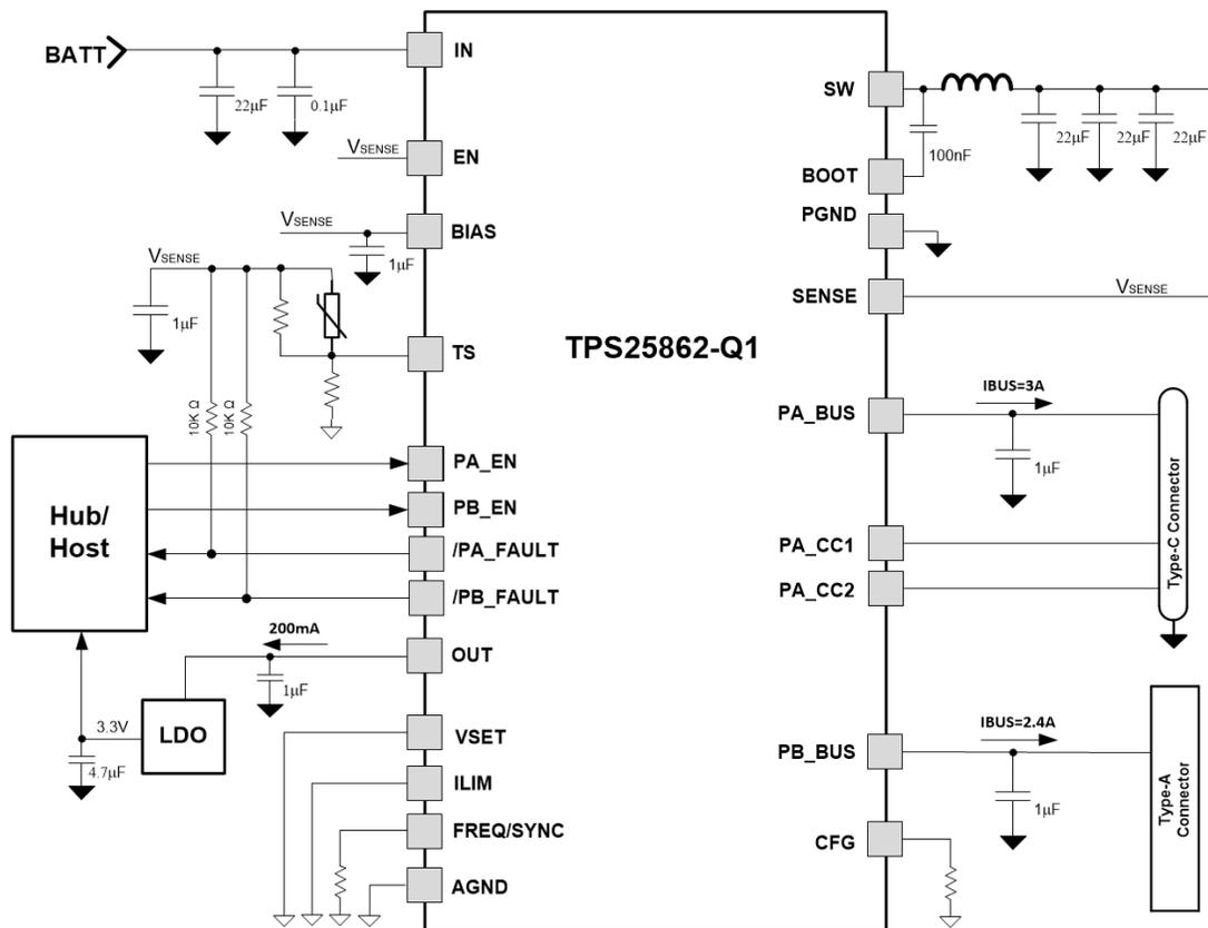
Figure 11-2. TPS25862-Q1 Typical Application Circuit for 2.1-MHz  $f_{sw}$
