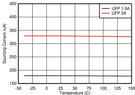
**Figure 8-23. CC Sourcing Current vs Junction Temperature**
