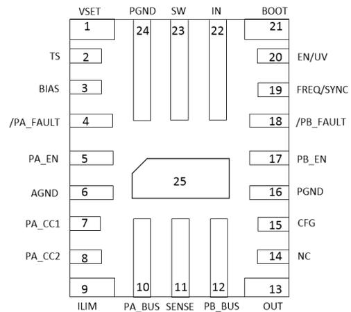
Figure 7-2. TPS25862 RPQ Package 25-Pin (QFN)
