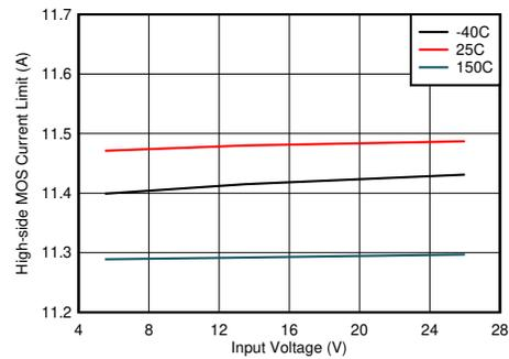
Figure 8-8. High-side Current Limit vs Input Voltage
