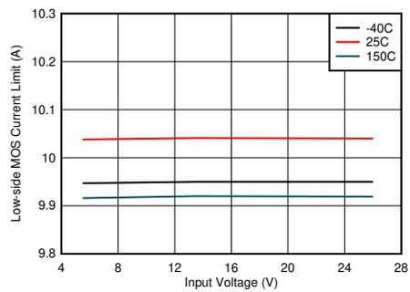
Figure 8-9. Low-side Current Limit vs Input Voltage
