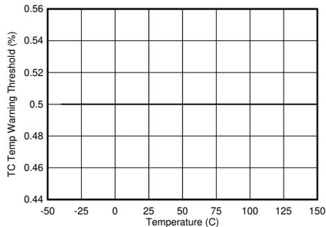
**Figure 8-24. TS Temperature Warning Threshold vs Junction Temperature**
