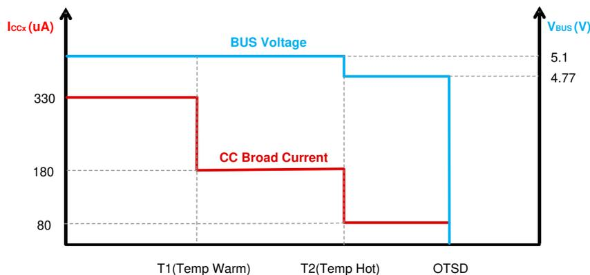
**Figure 10-17. TPS2586x-Q1 Behavior When Trigger Temp Warm/Hot Threshold**
