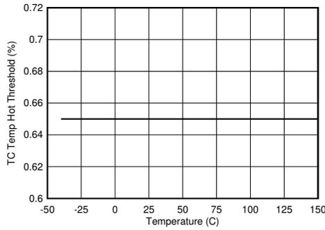
**Figure 8-25. TS Temperature Hot Threshold vs Junction Temperature**
