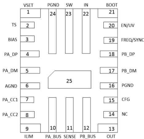
Figure 7-1. TPS25860 RPQ Package 25-Pin (QFN)
