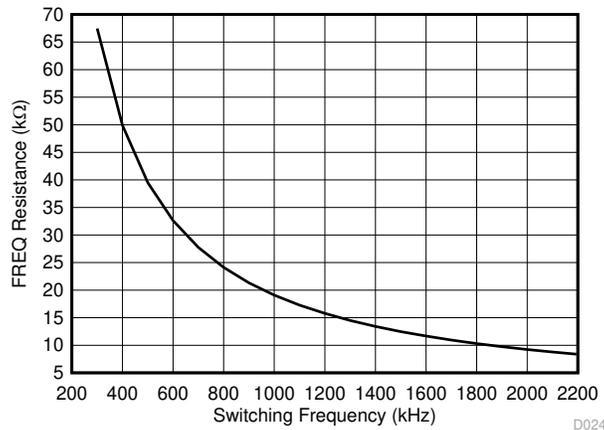
**Figure 10-3. FREQ Set Resistor vs Switching Frequency**
