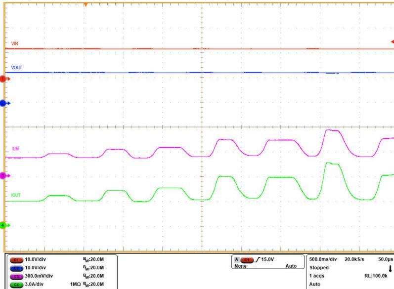
$V_{IN} = 12V$ ,  $C_{OUT} = 220\mu F$ ,  $R_{ILM} = 536\Omega$ ,  $I_{OUT}$  varied dynamically between 3A and 8A
