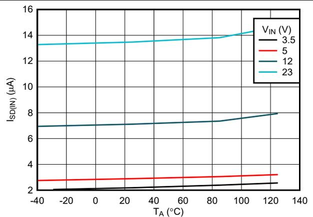
Figure 6-4. IN Shutdown Current vs Temperature
