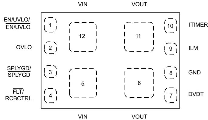
**Figure 5-1. YWP Package, 12-Ball PWCSPP (Top View)**
