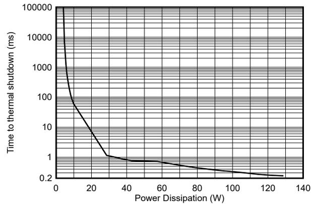
Figure 6-26. Time to Thermal Shut-Down During Inrush State
