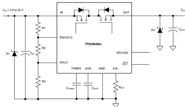
**Figure 8-25. Circuit Implementation With Optional Protection Components**
