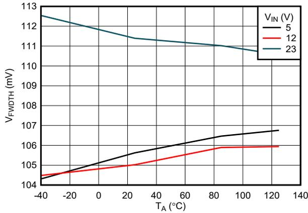
Figure 6-19. RCB - Forward Comparator Threshold vs Temperature
