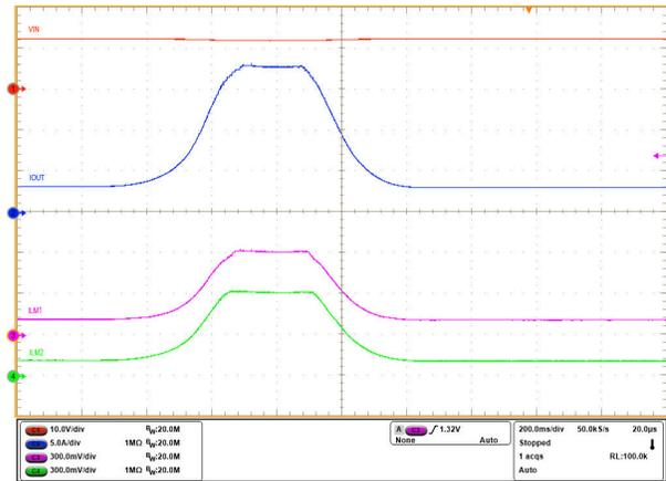
Figure 8-23. Parallel Devices Load Current During Steady State
