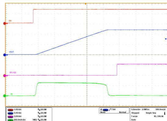
V<sub>IN</sub> = 12V, C<sub>OUT</sub> = 220μF, C<sub>dVdt</sub> = 10nF, V<sub>EN/UVLO</sub> stepped up to 2V
