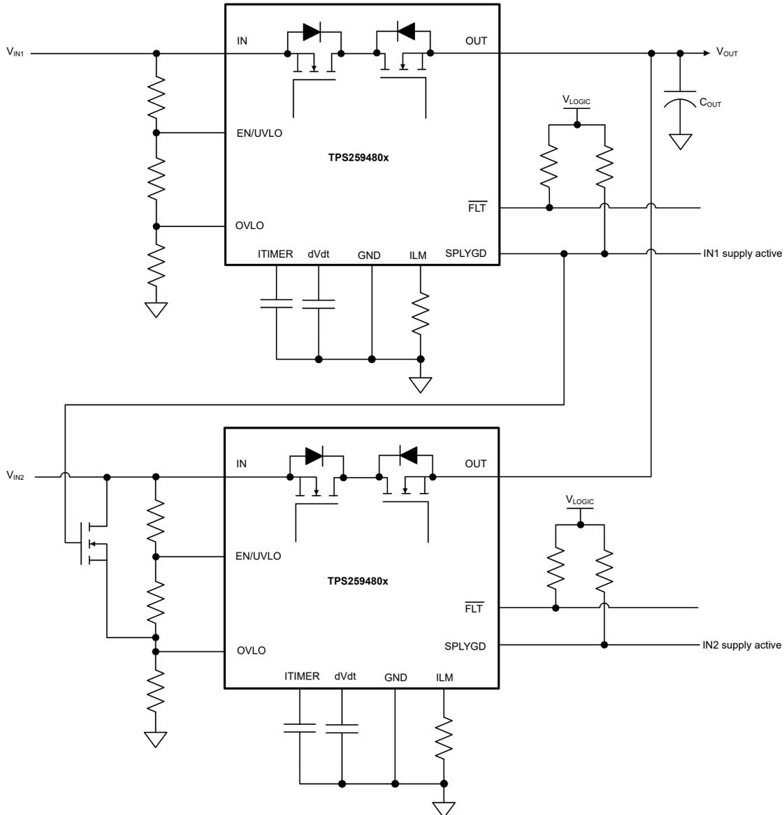
**Figure 8-19. Priority Power MUXing With 2 × TPS25948x - Option 2**
