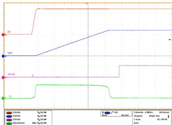
V<sub>EN/UVLO</sub> = 2V, C<sub>OUT</sub> = 220 μF, C<sub>dVdt</sub> = 10nF, V<sub>IN</sub> ramped up to 12V
