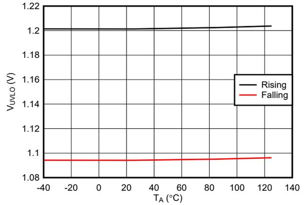
Figure 6-10. EN/UVLO FET Turn OFF Threshold vs Temperature
