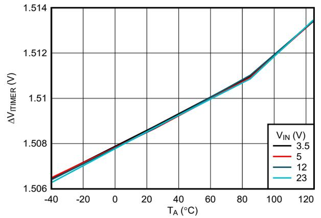
Figure 6-22. ITIMER Discharge Differential Voltage Threshold vs Temperature
