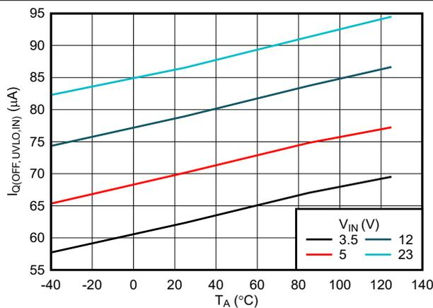
Figure 6-3. IN OFF state (UVLO) current vs Temperature
