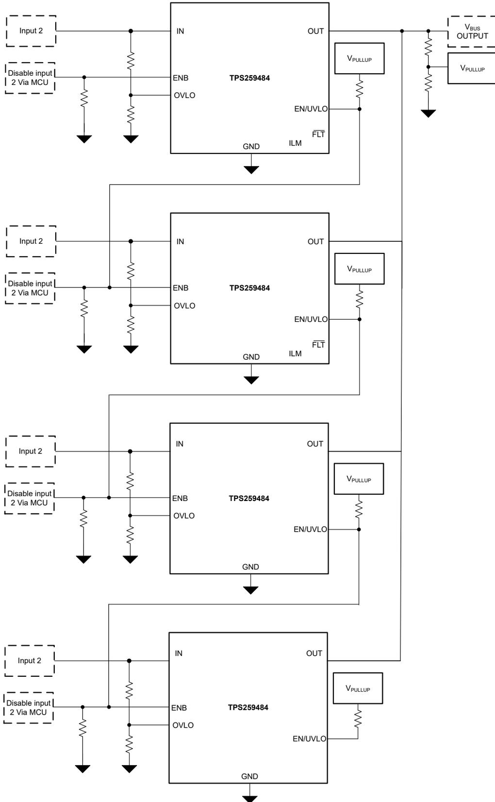
**Figure 8-4. Priority Power MUXing with 4 × TPS259484**
