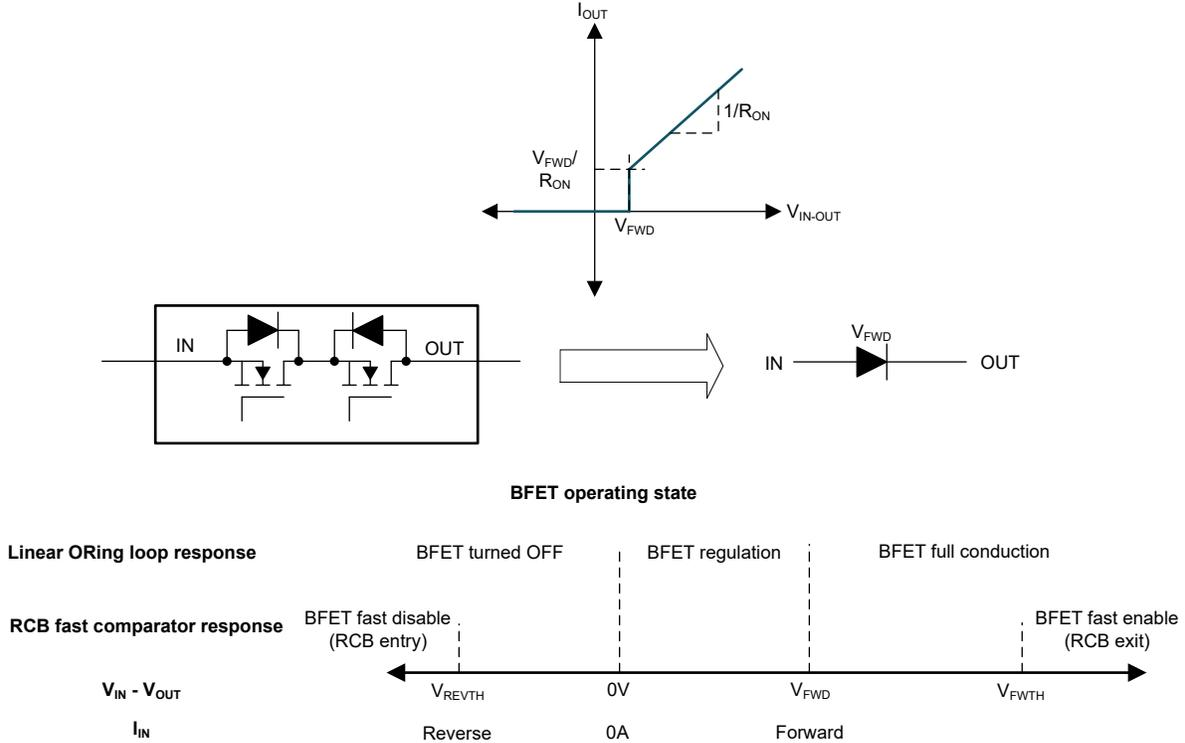
**Figure 7-12. Reverse Current Blocking Response**
