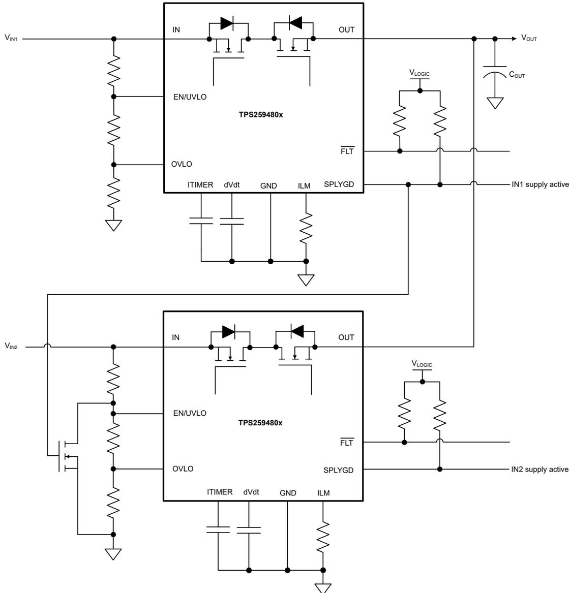
**Figure 8-20. Priority Power MUXing With 2 × TPS259480x - Option 3**
