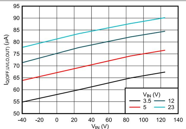
Figure 6-6. OUT OFF State (UVLO) Current vs Temperature
