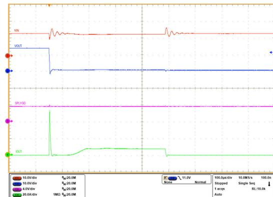
$V_{IN} = 12V$ ,  $I_{LIM}$  set to 9A,  $V_{EN}/UVLO = 2V$ ,  $I_{OUT}$  stepped from Open  $\rightarrow$  Short-circuit to GND
