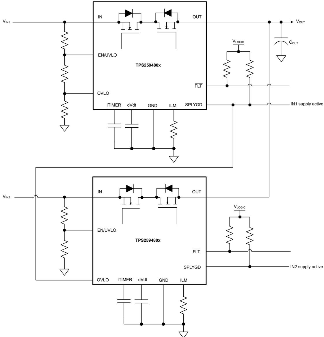
**Figure 8-16. Priority Power MUXing With 2 × TPS25948x - Option 1**
