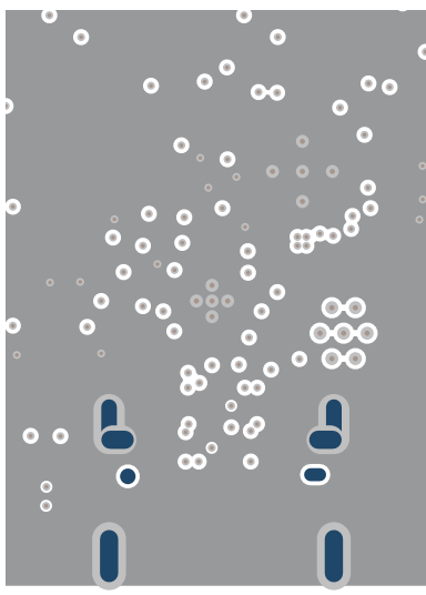
Figure 8-28. TPS26750 PCB Layout - GND Layer 2
