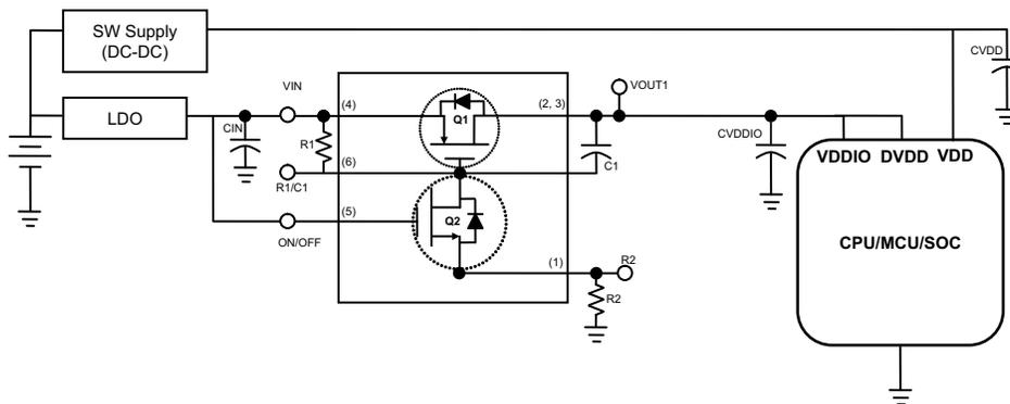
Figure 19. Power Sequencing Using TPS27081A
