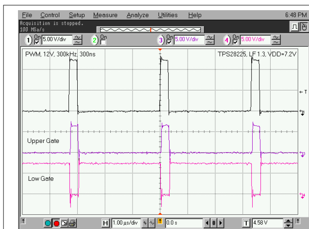
Figure 7-4. 12-V PWM Pulse at V_{DD} = 7.2\text{ V}
