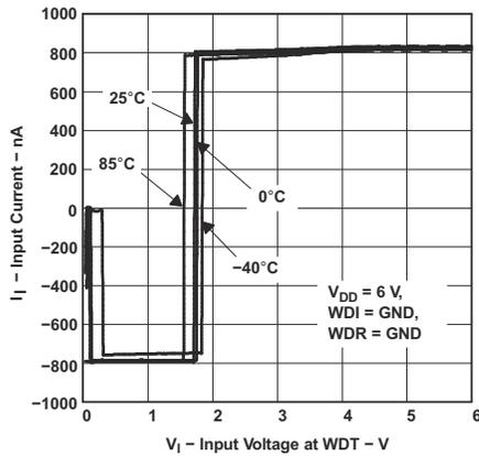
**Figure 6-4. Input Current vs Input Voltage at WDT**
