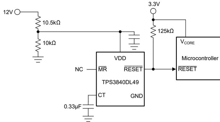
Figure 8-5. Fast Start Undervoltage Supervisor with Level-shifted Input
