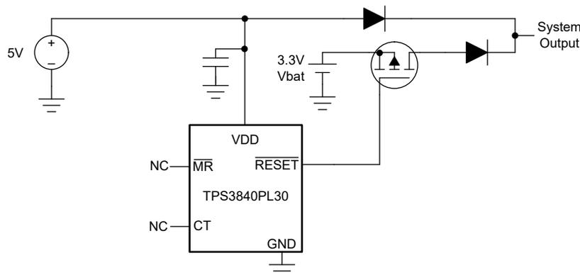
**Figure 8-6. Voltage Monitor with Back-up Battery Switchover Solution**
