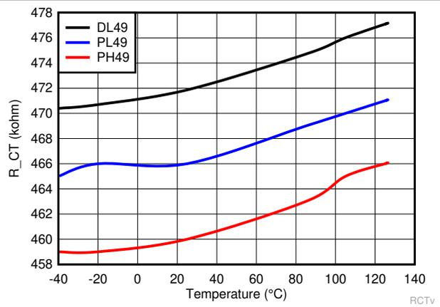
Figure 6-33. CT Pin Internal Resistance over Temperature
