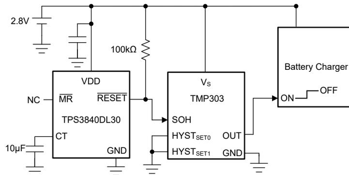
Figure 8-4. Overvoltage and Window Temperature Monitoring Solution
