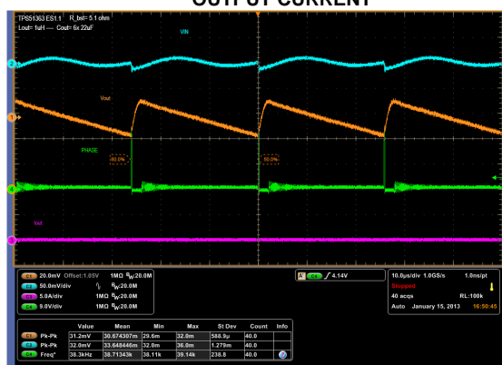
Figure 17. f = 400\text{kHz} , V_{IN} = 20\text{V} , I_{OUT} = 0.1\text{A}
