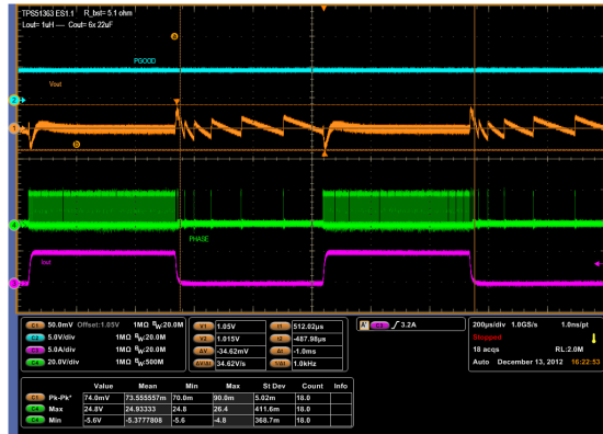
Figure 21. f = 400\text{kHz} , V_{IN} = 20\text{V} , I_{OUT} = 0-5\text{A}
