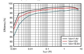
Efficiency Curve, V<sub>OUT</sub> = 5.1 V, PSM Mode
