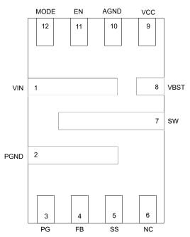
Figure 5-1. RJN Package 12-Pin VQFN-HR Top View
