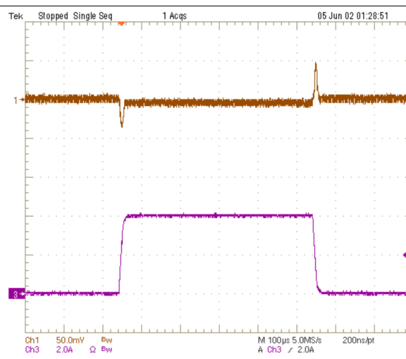
Figure 16. Load Transient Response
