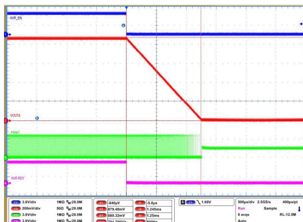
Figure 8-9. Soft-stop channel A (0 ms TOFF_DELAY)
