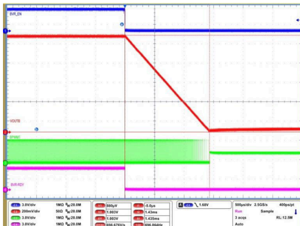
Figure 8-20. Soft-stop channel B (0 ms TOFF_DELAY)
