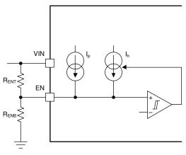
Figure 7-2. Adjustable UVLO Using EN
