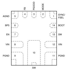
Figure 5-1. 14-Pin VQFN-HR RPY Package (Top View)
