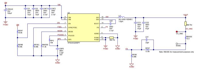
Figure 8-21. 12-V Input, 1.8-V Output, 1.5-MHz Schematic
