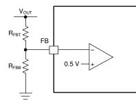
Figure 7-3. FB Resistor Divider
