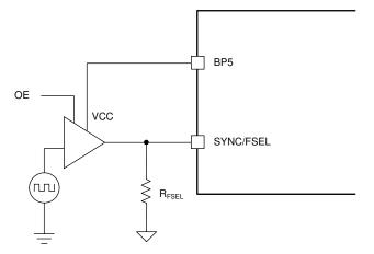
Figure 7-5. Interfacing the SYNC/FSEL Pin with a Buffer
