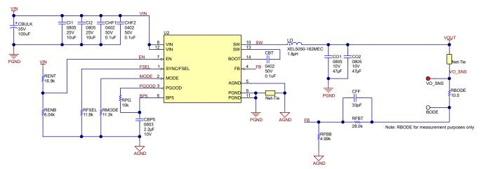
Figure 8-1. 12-V Input, 3.3-V Output, 1.0-MHz Schematic
