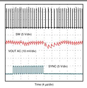
Figure 7-4. Clock Synchronization Transitions
