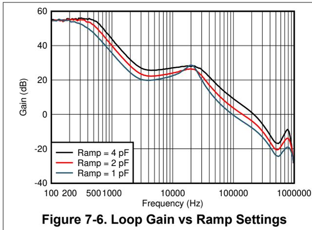
Figure 7-6. Loop Gain vs Ramp Settings
