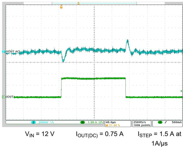
Figure 8-8. Load Transient
