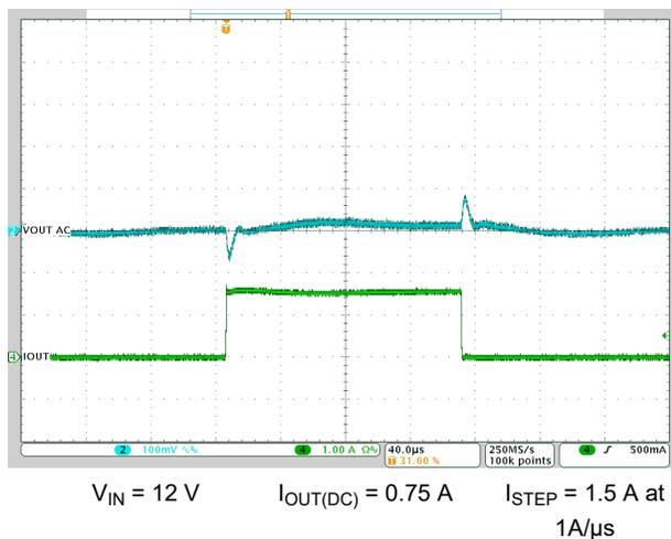
Figure 8-26. Load Transient
