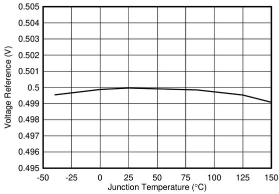
**Figure 6-7. Regulated FB Voltage vs Junction Temperature**
