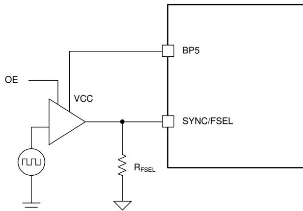
Figure 7-5. Interfacing the SYNC/FSEL Pin with a Buffer
