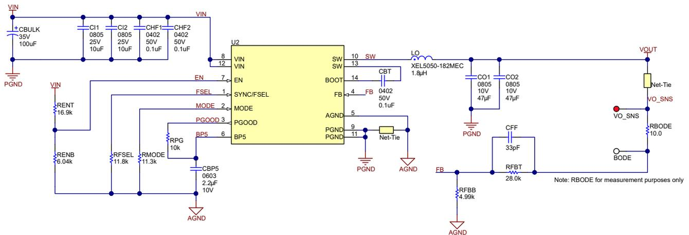
Figure 8-1. 12-V Input, 3.3-V Output, 1.0-MHz Schematic
