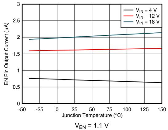
**Figure 6-8. EN Pin Current vs Junction Temperature**
