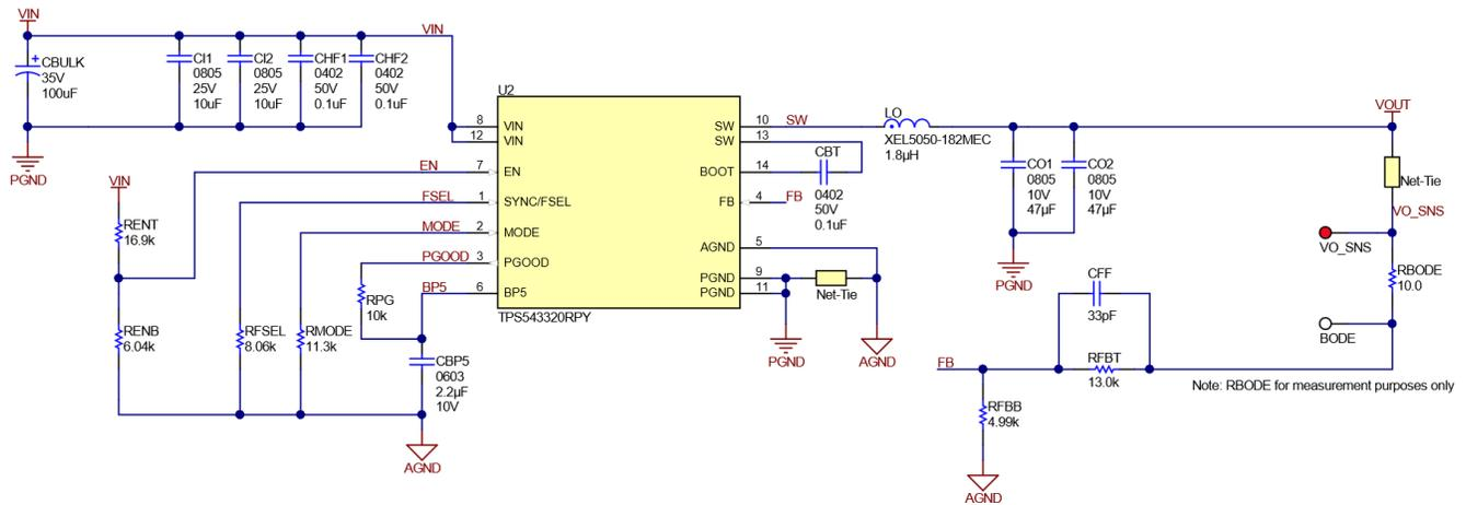
Figure 8-21. 12-V Input, 1.8-V Output, 1.5-MHz Schematic
