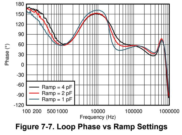
Figure 7-7. Loop Phase vs Ramp Settings
