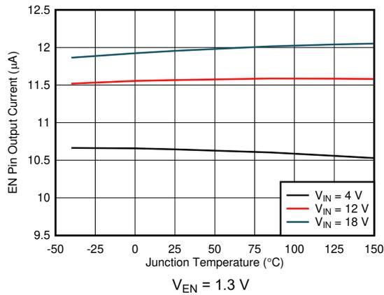
**Figure 6-9. EN Pin Current vs Junction Temperature**
