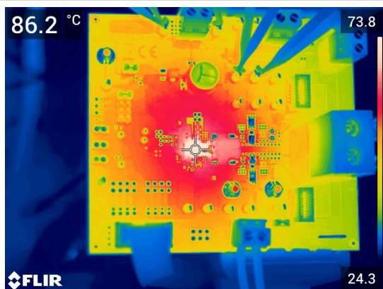
Figure 8-21. Thermal Characteristics, 600 kHz FCCM, Internal LDO, 35-A Load
