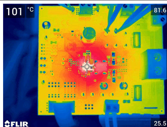
Figure 8-26. Thermal Characteristics, 1.2-MHz FCCM, External 5-V Bias, 35-A Load
