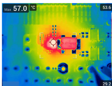
Figure 8-10. Thermal Characteristics, 800kHz FCCM, External 5V Bias, 25A Load
