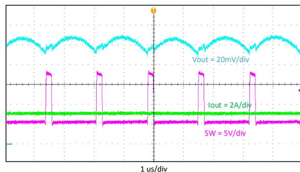
**Figure 9-7. Output Voltage Ripple,  $i_{out} = 3\text{ A}$**
