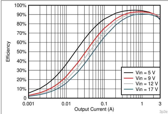
Figure 7-13.  $V_{OUT} = 3.3\text{-V}$  Efficiency,  $L = 3.3\ \mu\text{H}$
