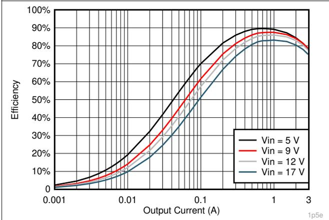
**Figure 7-11.  $V_{OUT} = 1.5\text{-V}$  Efficiency,  $L = 2.2\ \mu\text{H}$**
