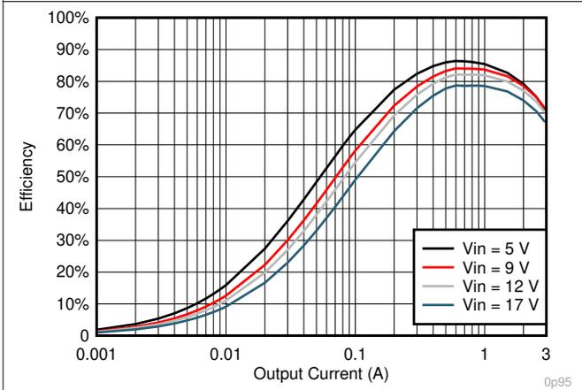
**Figure 7-9.  $V_{OUT} = 0.95\text{-V}$  Efficiency,  $L = 1.5\ \mu\text{H}$**
