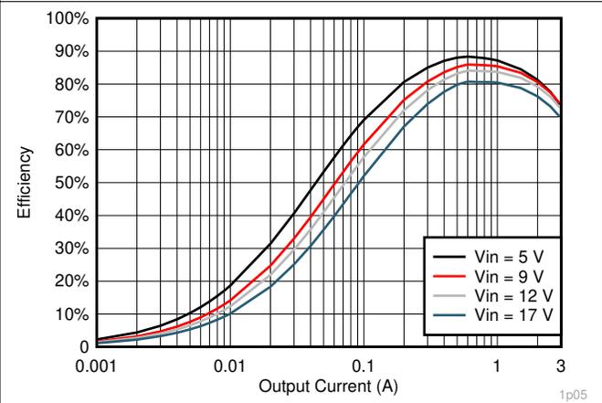
**Figure 7-10.  $V_{OUT} = 1.05\text{-V}$  Efficiency,  $L = 1.5\ \mu\text{H}$**
