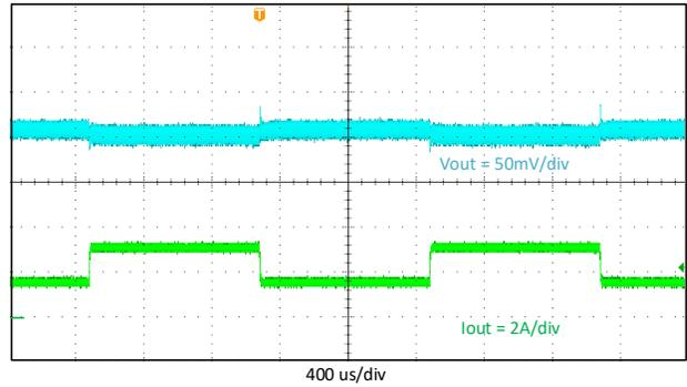
**Figure 9-9. Transient Load Response, Iout = 1.5 to 3 A**
