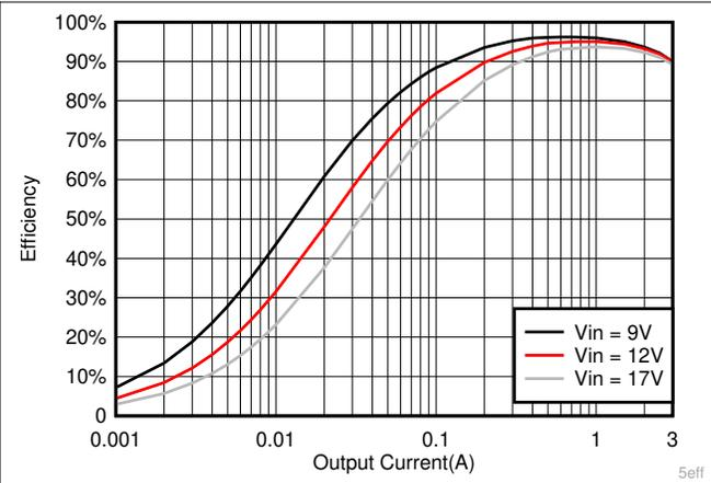
Figure 7-14.  $V_{OUT} = 5\text{-V}$  Efficiency,  $L = 4.7\ \mu\text{H}$
