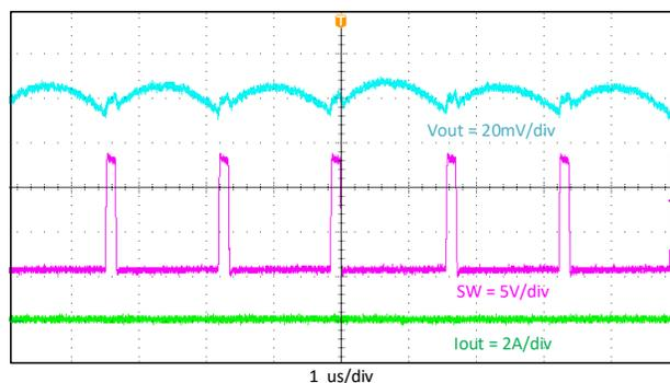
**Figure 9-6. Output Voltage Ripple,  $i_{out} = 10\text{ mA}$**
