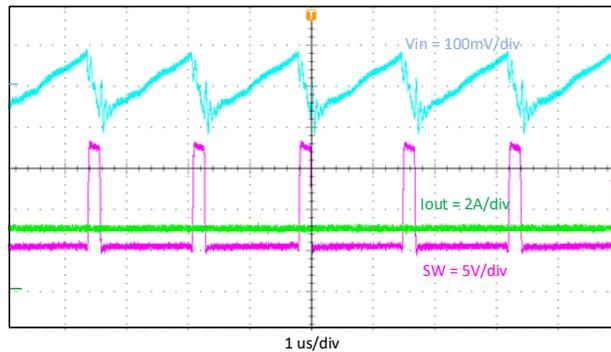
**Figure 9-4. Input Voltage Ripple  $i_{out} = 3\text{ A}$**
