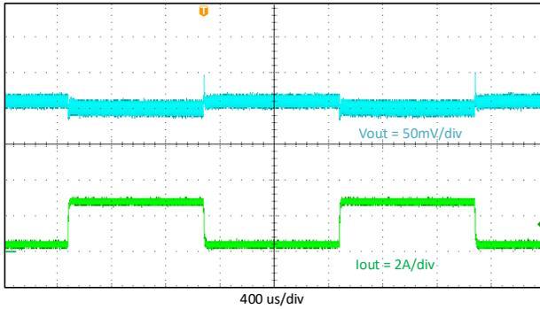
**Figure 9-8. Transient Load Response, Iout = 0.3 to 2.7 A**
