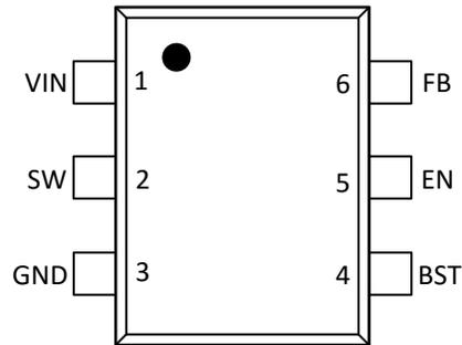
**Figure 6-1. 6-Pin SOT563 DRL Package (Top View)**
