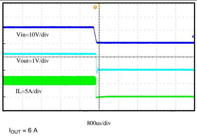
Figure 28. Shut Down Relative to V<sub>IN</sub> Falling
