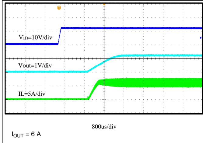
Figure 27. Start Up Relative to V<sub>IN</sub> Rising
