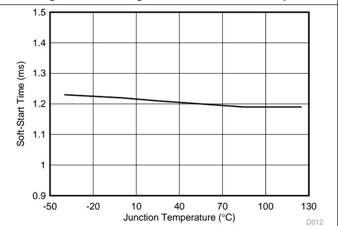
Figure 12. Soft-Start Time vs Junction Temperature
